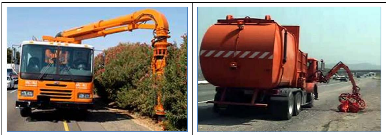
Figure 1. Automated Road Debris Vacuum (Left) and Litter Bag/Debris Vehicle (Right) (Strong and Valdes-Vasques, 2014).
