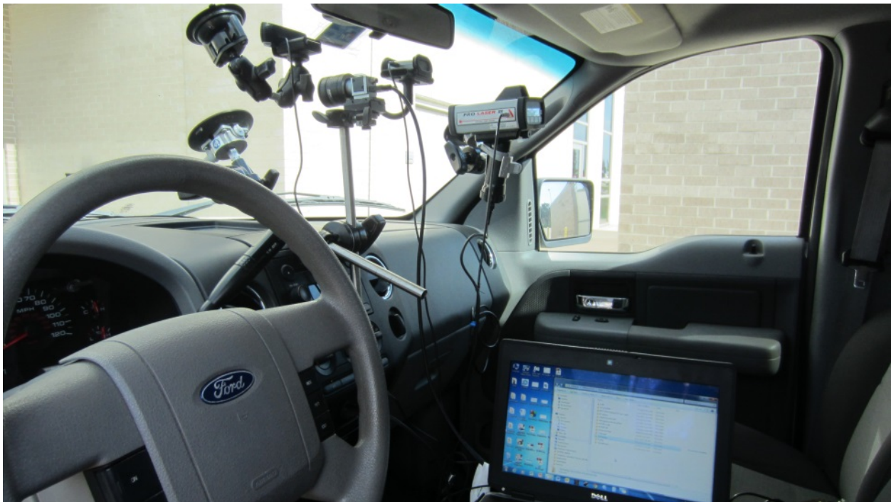
Figure 24. Setup for System Developed in Previous Study to Estimate Distance to a Leading Vehicle.
