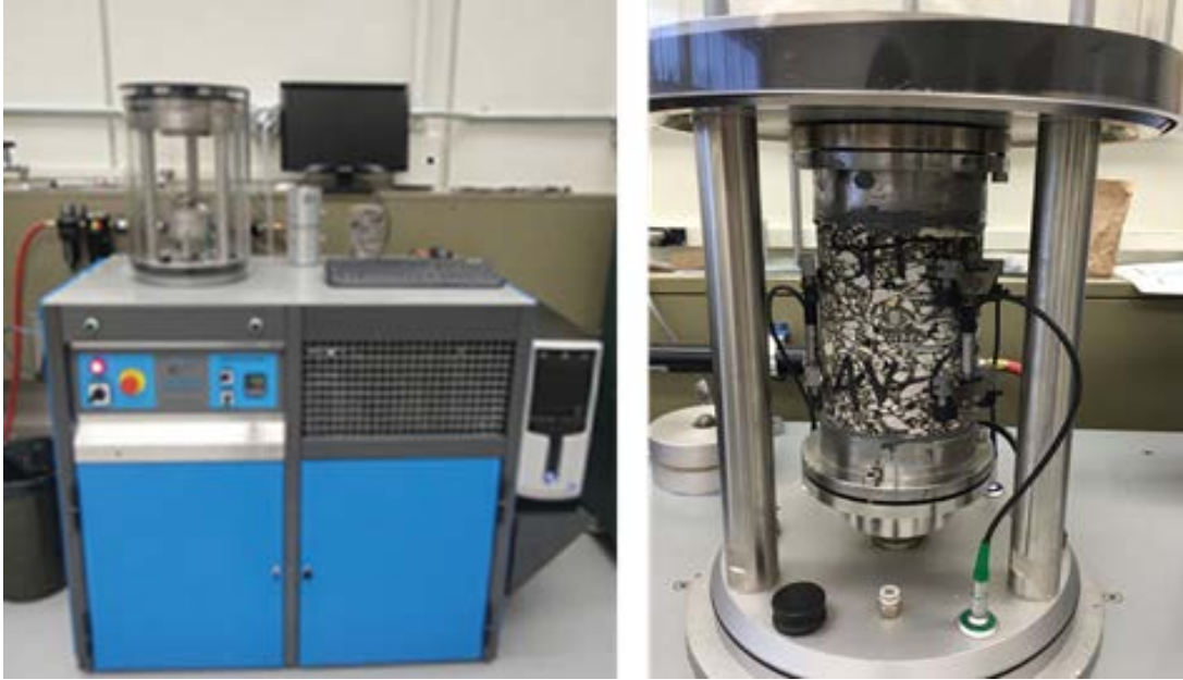
Figure VII-3. The AMPT Setup and S-VECD HMA Sample.
