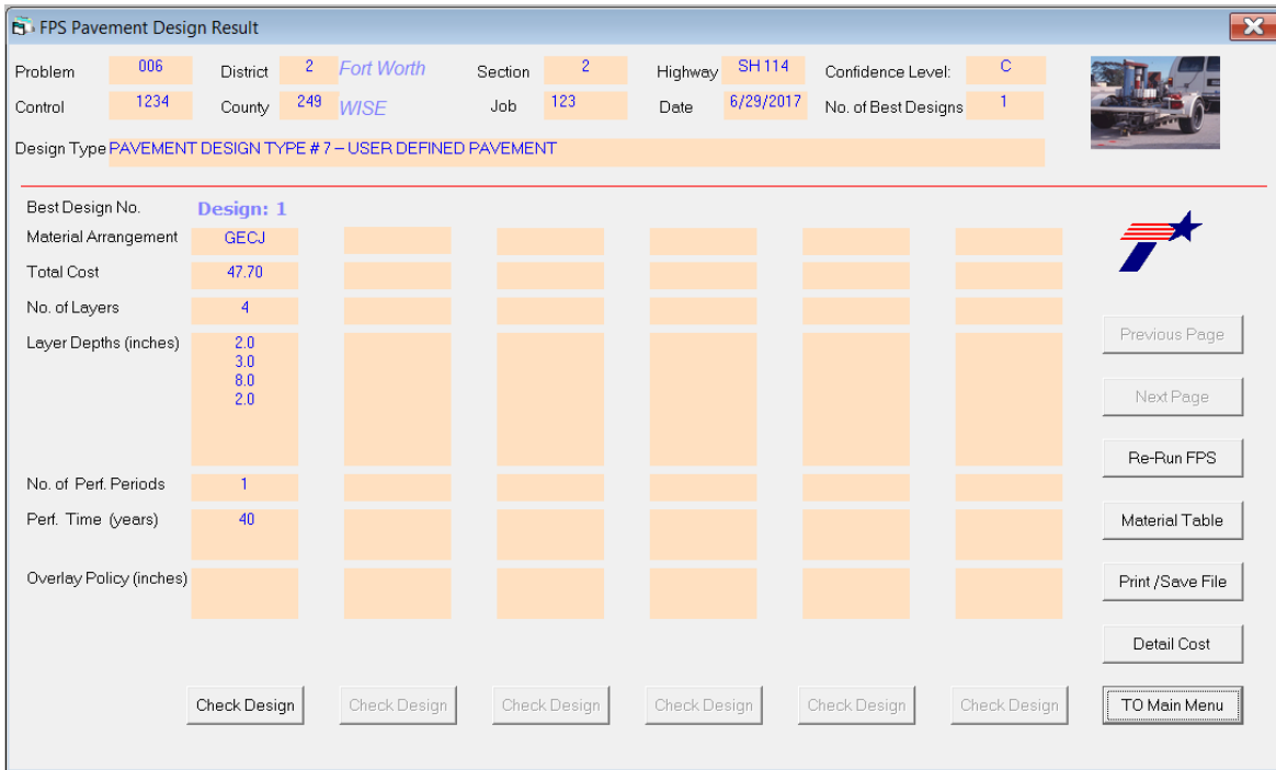
(a) FPS Pavement Design Result.
