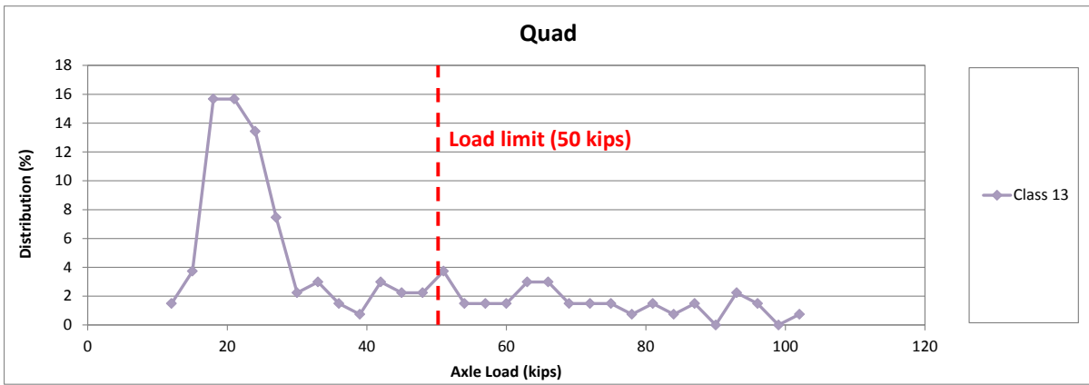
Figure II-2. Axle Load Spectra from WIM Station (SH 114 FTW, 2011) (Continued).
