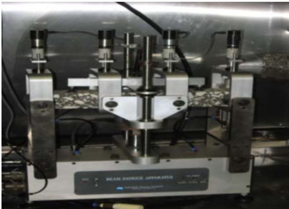
Figure VII-1. The Bending Beam Fatigue Test Apparatus and HMA Specimen.
