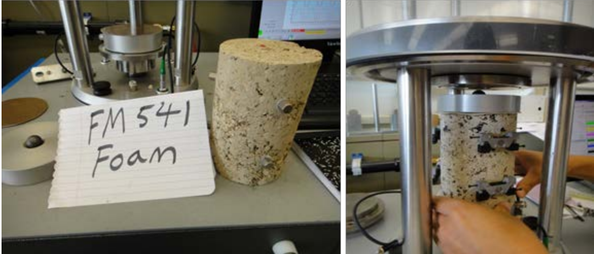
Figure 27. Dynamic Modulus Testing of Stabilized Materials (FDR).
