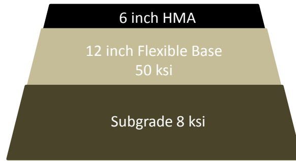
Figure 10. A Typical Pavement Structure.
