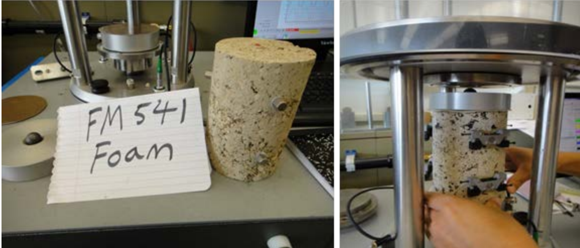
Figure 20. Dynamic Modulus Testing of Asphalt Stabilized Material.
