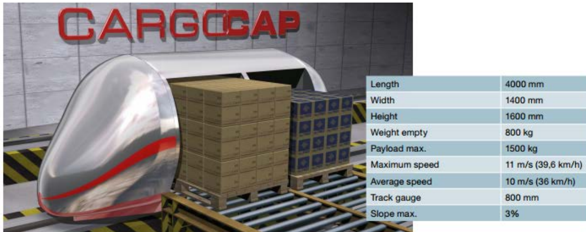
Figure A-40. CargoCap Prototype and Specifications.
