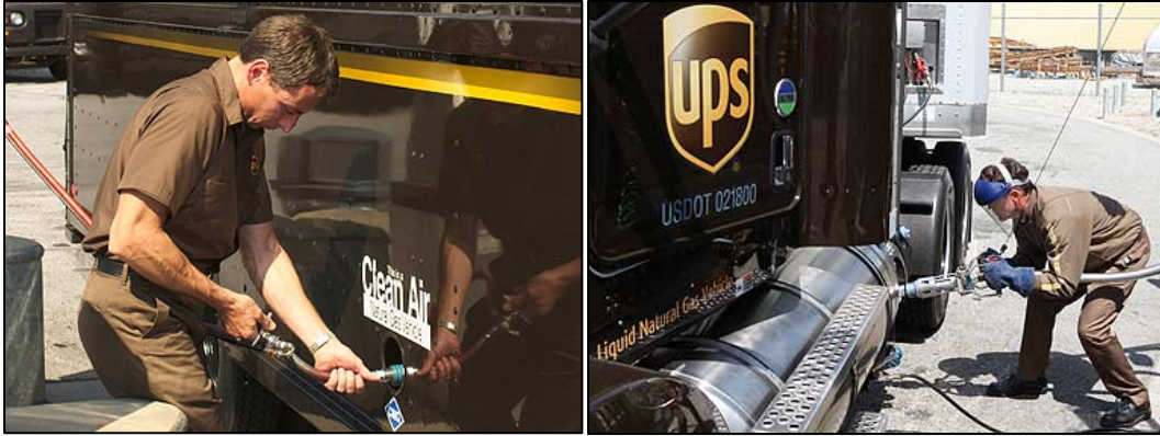
Figure A-17. Refueling—Left: CNG truck; Right: LNG truck
