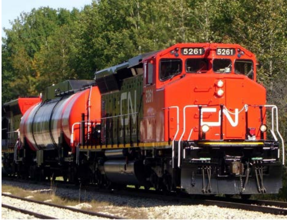
Figure A-7. Canadian National ElectroMotive Diesel SD40-2 locomotives with tender converted to use natural gas fuel with diesel pilot operated from September 2012 to November 2013 between Edmonton and Ft. McMurry, Alberta, Canada.
