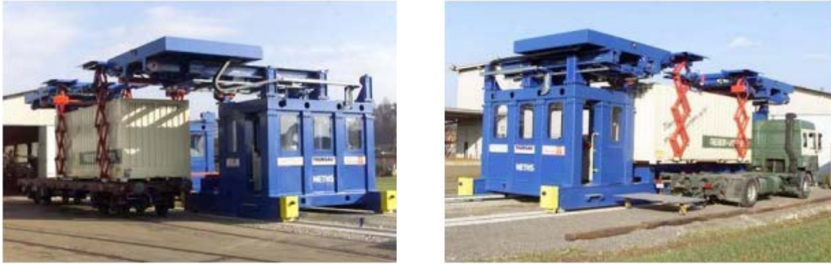
Figure A-34. Pictures of the Neuweiler Tuchschmid Horizontal Transshipment System (NETHS).
