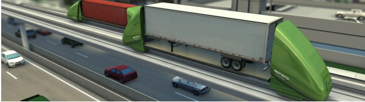
Figure A-1. Conceptual Drawing of the Freight Shuttle System by Linear Induction Propulsion.
