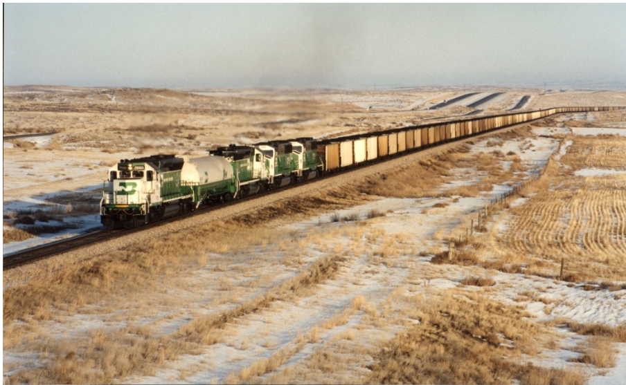
Figure A-6. The first worldwide LNG fueled locomotive to operate in regular-revenue coal-train service from September 1991 to February 1996 between Decker, Montana, and Allouez Coal Dock, Superior, Wisconsin.
