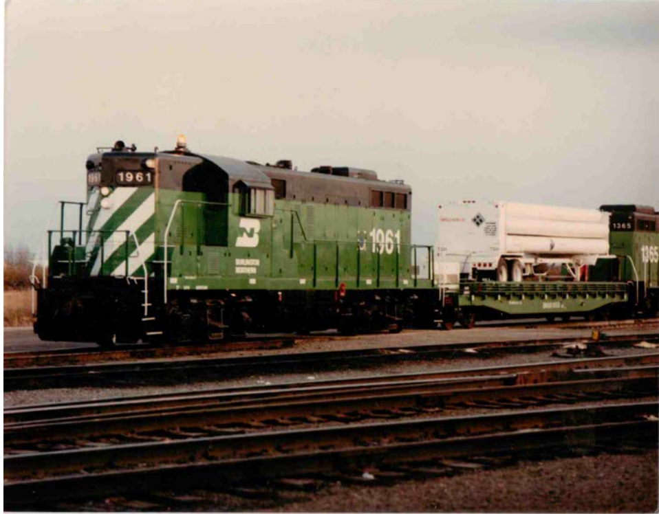
Figure A-5. The first worldwide natural-gas-fueled locomotive to operate in revenue service from October 1984 to May 1988 between Minneapolis, Minnesota, and Superior, Wisconsin.
