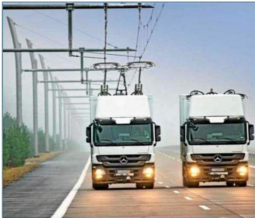
Figure A-18. Side-by-Side Picture of Dual-Mode Truck in Electric and Diesel Modes.
