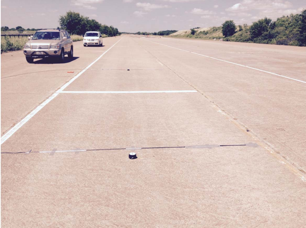
Figure 54. Photo of Magnetometers and Tapeswitches as Tested at Riverside.
