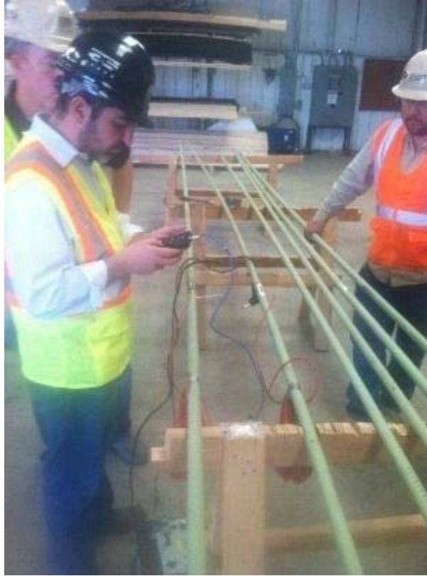
Figure 215. Testing the Gauges before Installing the Aluminum Cover.
