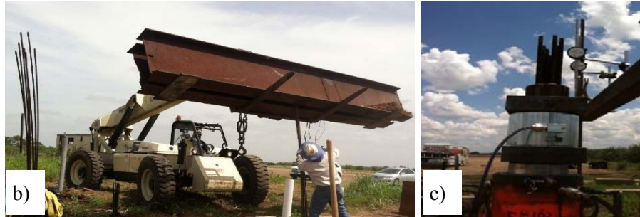
Figure 65. Load Test Setup in July 2013: a) Photo of Pullout Test, b) Placing the Reaction Beam, and c) Load Cell and Dial Gauges.
