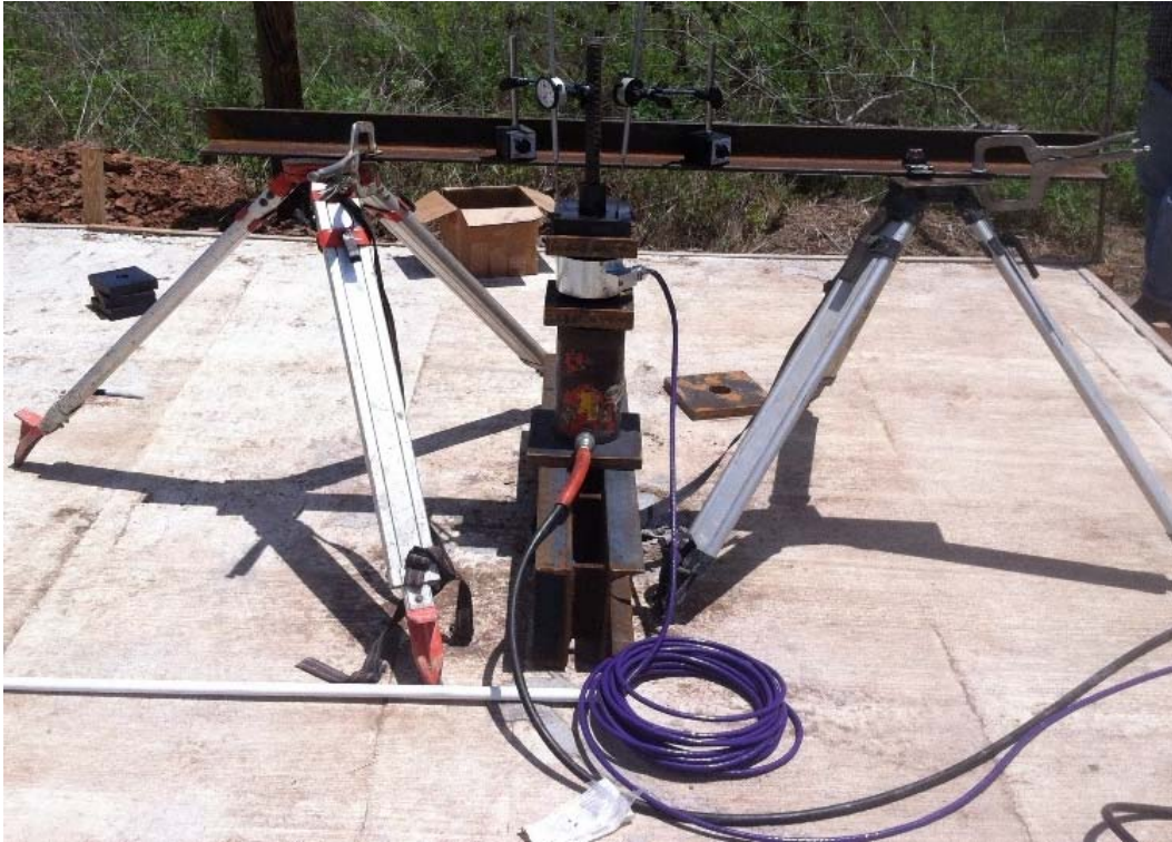
Figure 108. Load Test Setup for the Nails on Concrete Slab (i.e., Nails N1 to N6).
