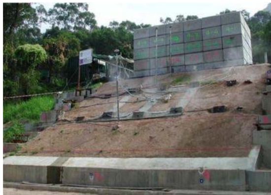
Figure 31. Soil Nail Slope with Surcharge (after Li et al., 2008).
