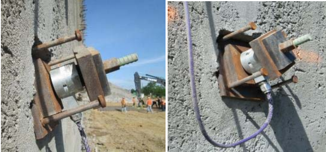
Figure 238. Load Cell Setup at the Nail Head.
