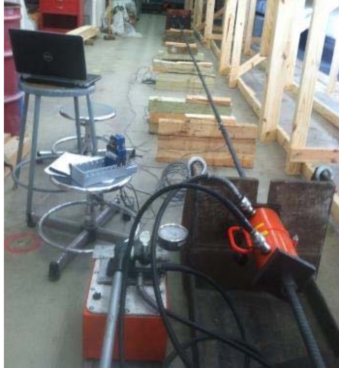
Figure 156. Adopted Setup for the Load Tests on Instrumented Nails Performed at TAMU prior to Shipping the Nail Bars to the Beaumont Site.
