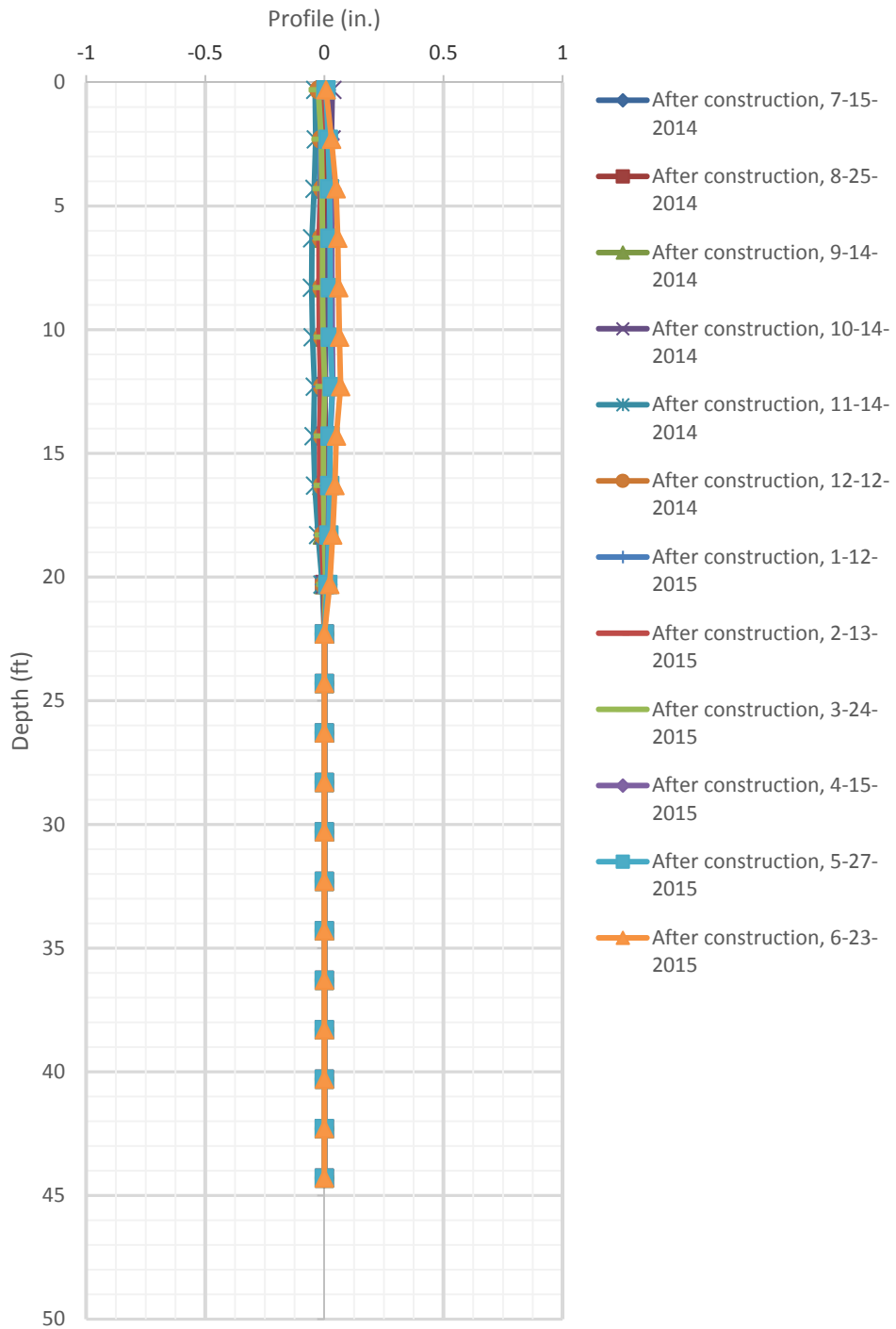
Figure 193. Lateral Displacements of the Soil Profile at 3 Ft behind the Facing of the Wall at Station 2+00 after Construction.
