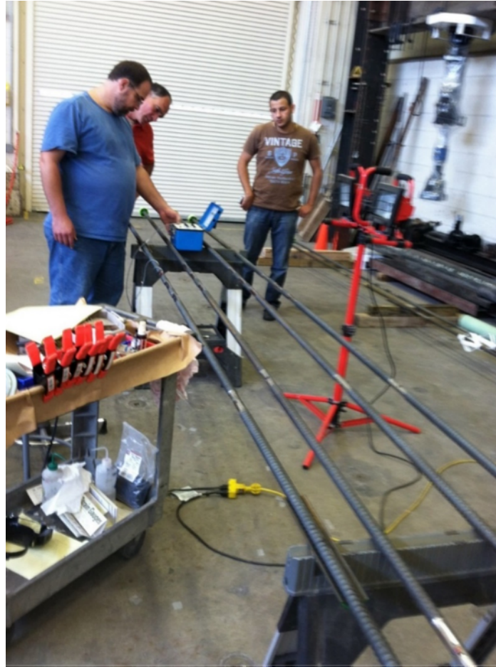
Figure 95. Testing the Strain Gauges with Vishay’s P3 Strain Indicator prior to Shipping to the NGES-TAMU Clay Site.
