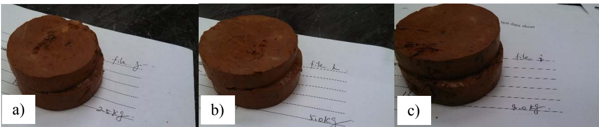
Figure 283. Photos of Samples (Depths 13 to 15 Ft Borehole N1) at Failure a) at Ratio of 1, b) at Ratio of 2, and c) at Ratio of 3.
