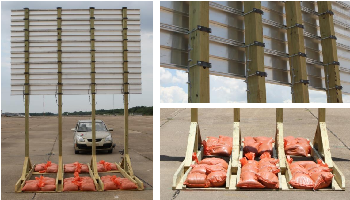
Figure 2. Wooden Skid-Mounted Sign Support System.
