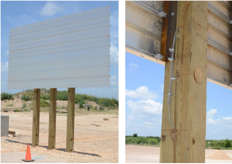
Figure 1. Wooden Direct Embedded Sign Support System.
