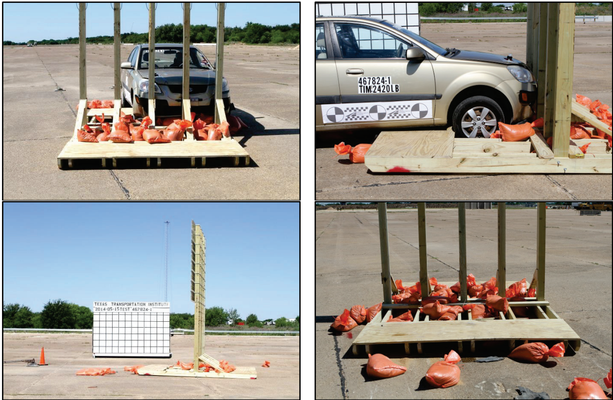
Figure 4.4. Skid-Mounted Support System for Temporary Guide Signs after Test No. 467824-1.
