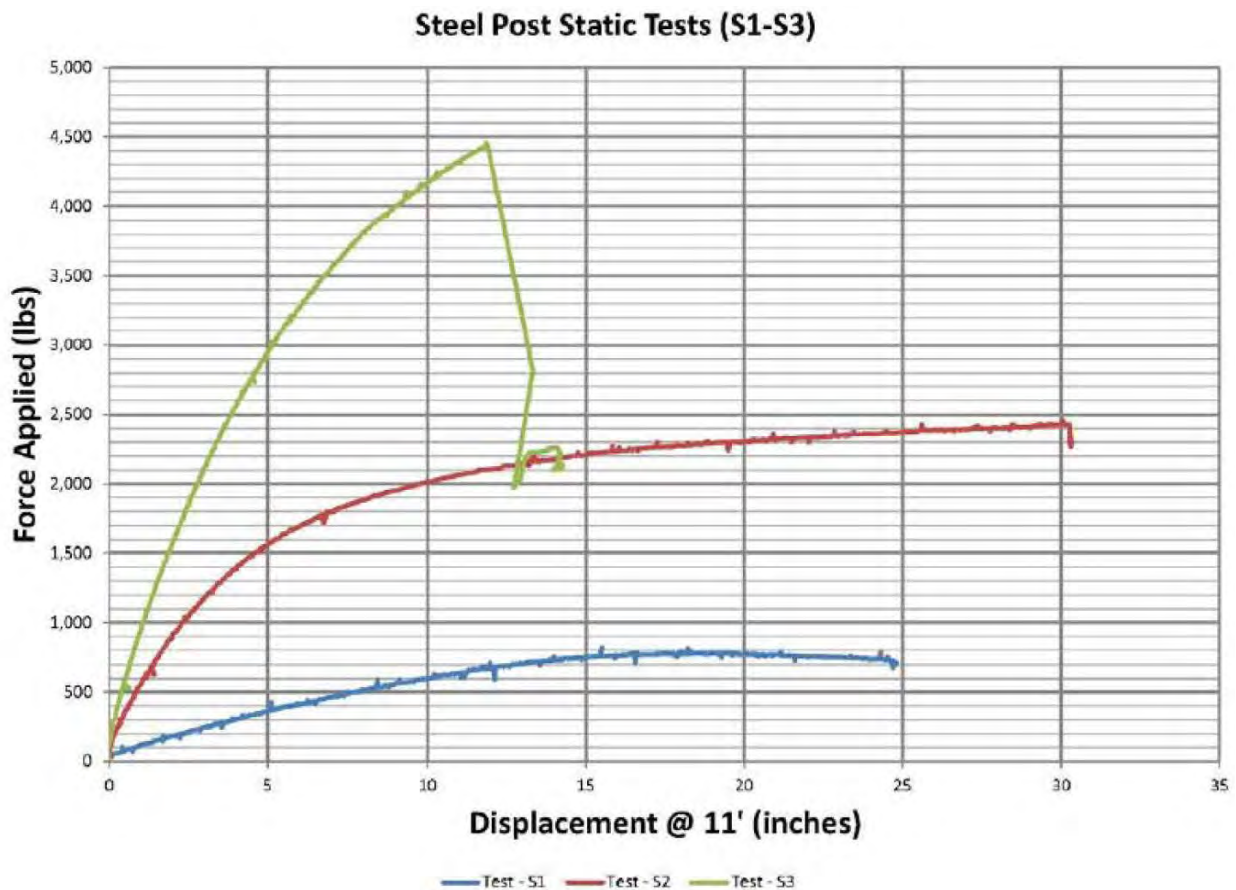
Figure 5.1. Static Test Results for S3×5.7 (Test S1), W6×9 (Test S2), and W8×18 (Test S3).
