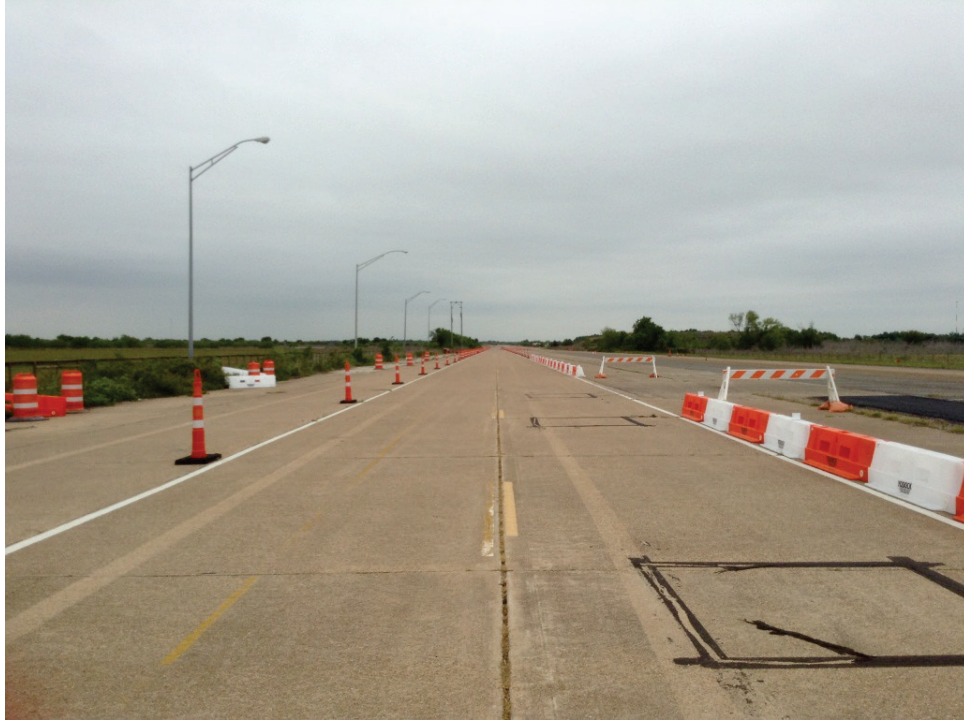
Figure A-31. Treatment 9: 18-Inch LCDs on Main Lane with 36-Inch Type I Barricades on Driveway.
