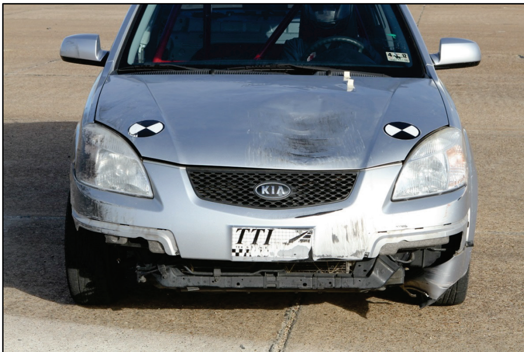
Figure 1.3. Kia Rio ( MASH Test Vehicle) after 100 Impacts.
