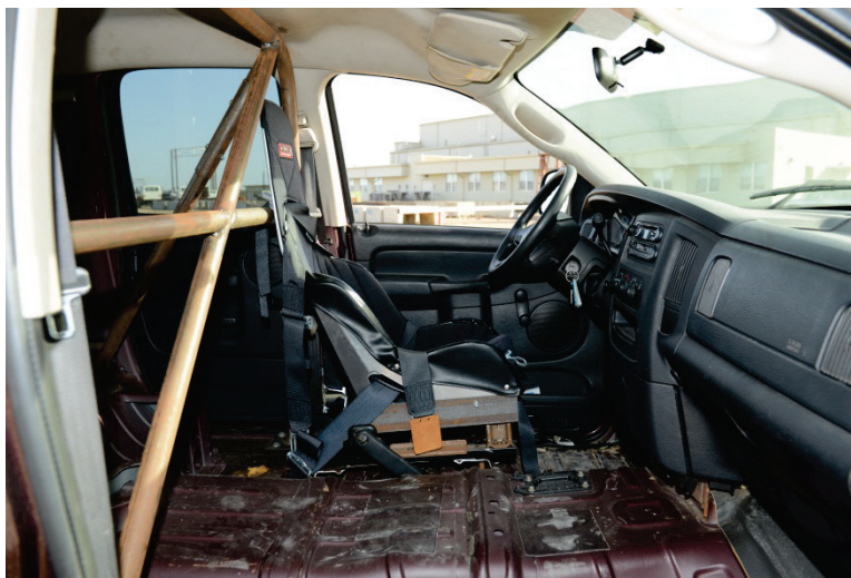
Figure 4.6. 2270P Vehicle Modifications.
