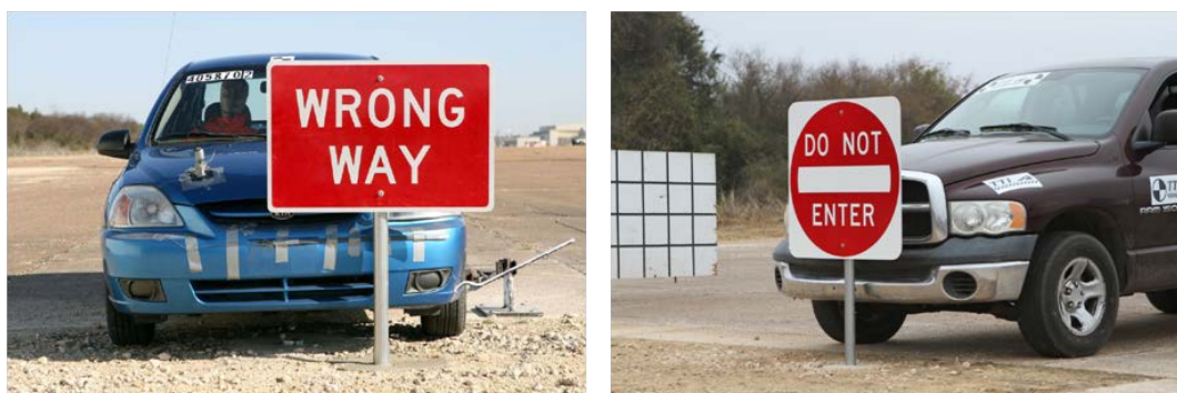
Figure 2. Crash Testing of Lowered Sign Mounts.
