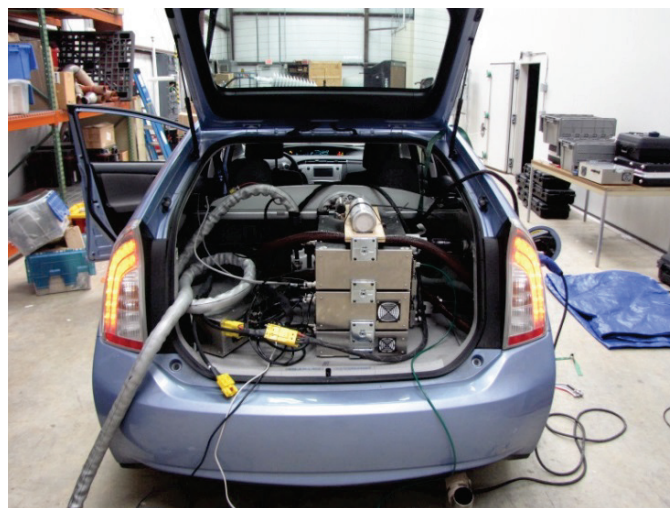
Figure 14. PEMS Equipment in Test Vehicle.
