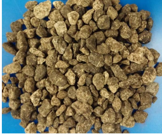
Figure 7. LRA Aggregate Precoated with Flux Oil.
