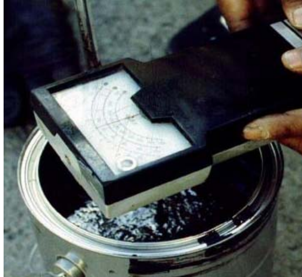
Figure 8. Field Viscosity Testing of A-R Binder.
