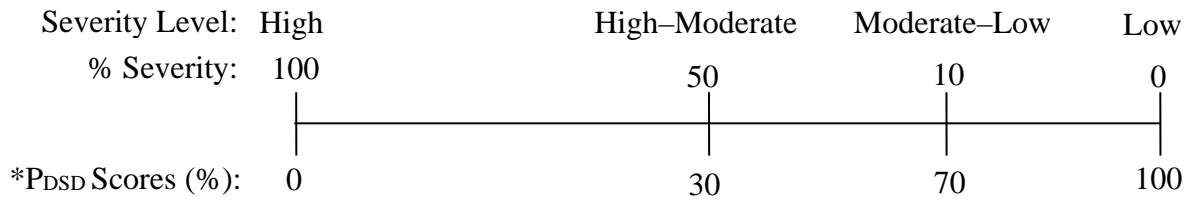
Figure 52. SCI Distress Evaluation and Scores – DSD.
