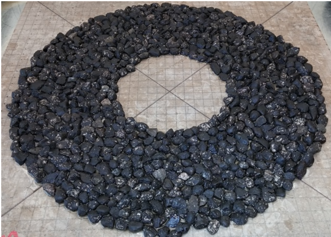
Figure 44. Test Specimen Fabrication Using Ward Co. Gravel.
