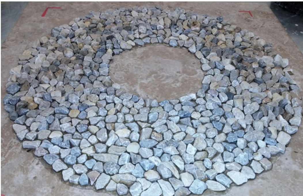
Figure 42. Test Specimen Fabrication Using Perch Hill Limestone.
