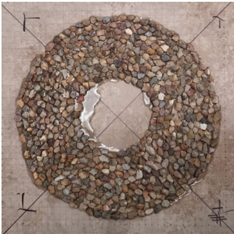
Figure 38. Test Specimen Fabrication Using Fordyce Gravel.
