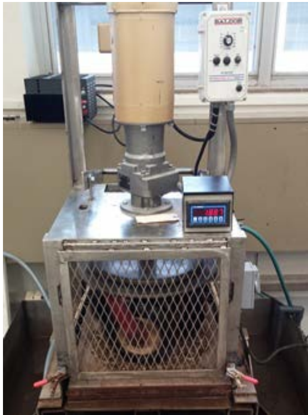
Figure 37. Three-Wheel Polisher and Circular Track Meter.
