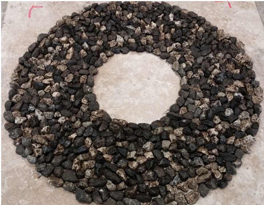
Figure 46. Test Specimen Fabrication Using Leach Pit Limestone.
