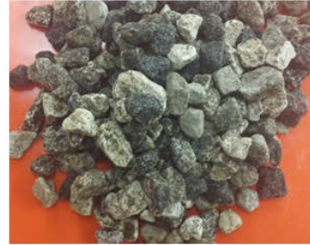
Aggregates before binder extraction
