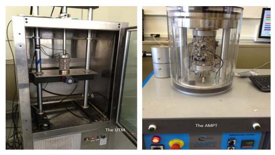
Figure 4-2. Comparison of the Environmental Chambers.
