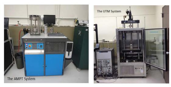
Figure 4-1. Pictures of the AMPT and UTM Units.
