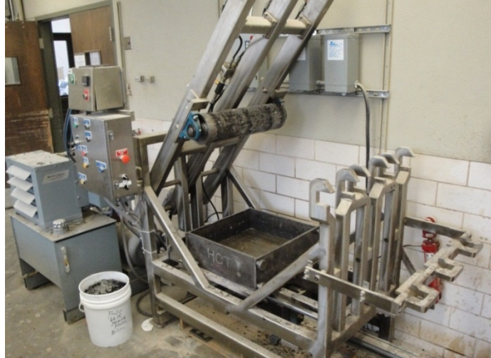
Figure 3.2. PMW Linear Compactor for Molding Slabs.
