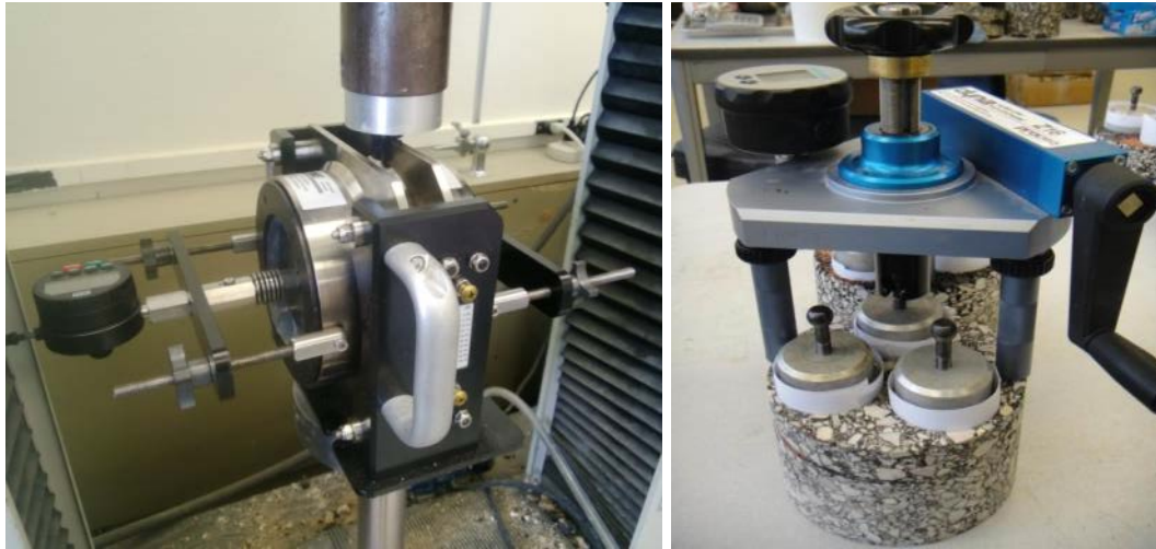
Figure G.3. Bond Strength Test Devices: Shear Test (Left) and Pull-Off Test (Right).
