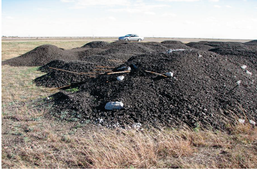
Figure 19. Contaminated RAP Stockpile.
