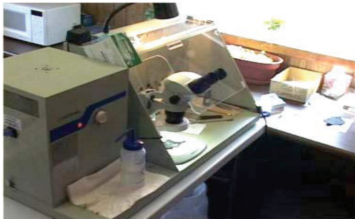
Figure 23. Setup for Asbestos Testing (13).
