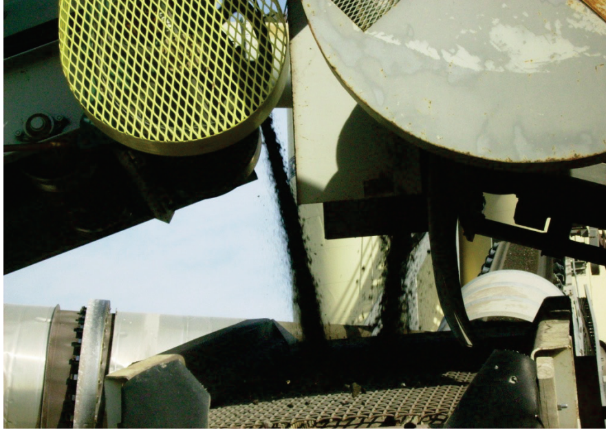
Figure 28. Vibratory Scalping Screen (19).
