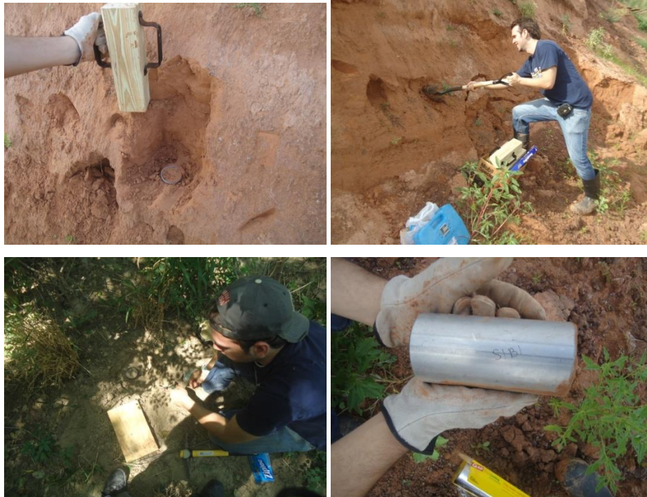
Figure 24: Obtaining samples with muffler tube
