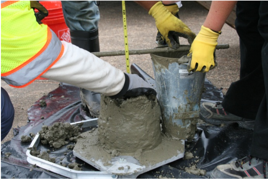
Figure B.28. Slump Measurement (CC).
