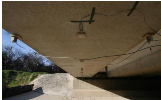
(b) Strain Gage and String Potentiometer
