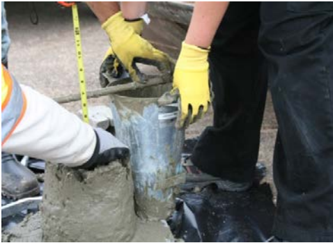
(c) Slump Test
