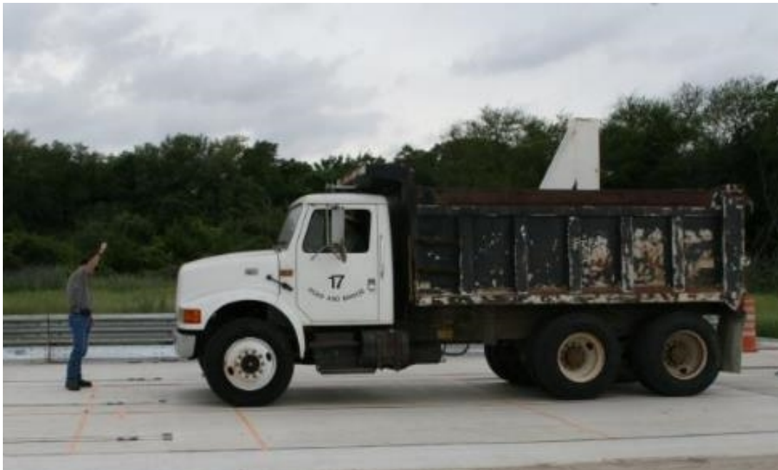
Figure 4.16. Static Loading with Dump Truck.
