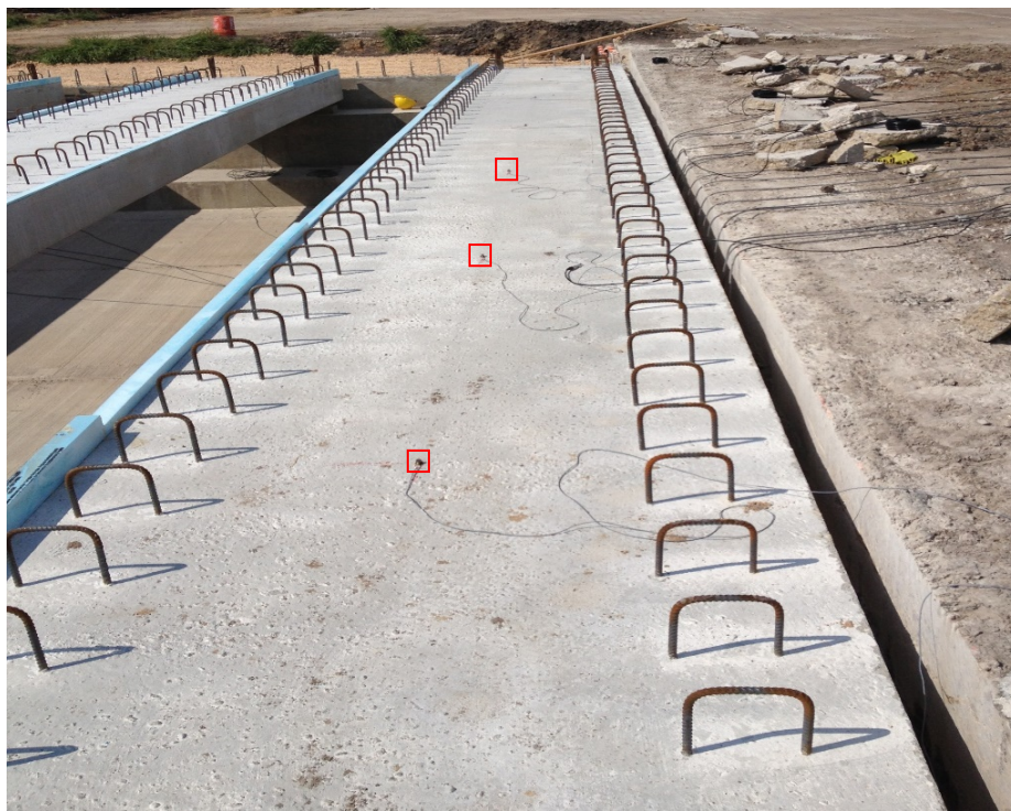
Figure 4.7. Accelerometer Positions for Individual Beam Test.
