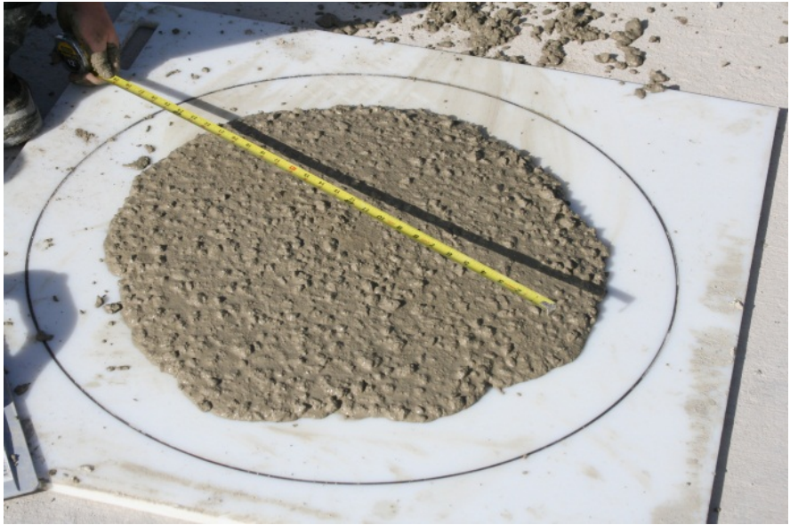
Figure B.29. Slump Measurement (SCC).
