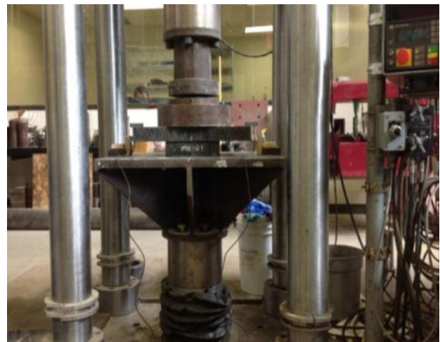
(b) 9 in. by 9 in. Bearing Pad
