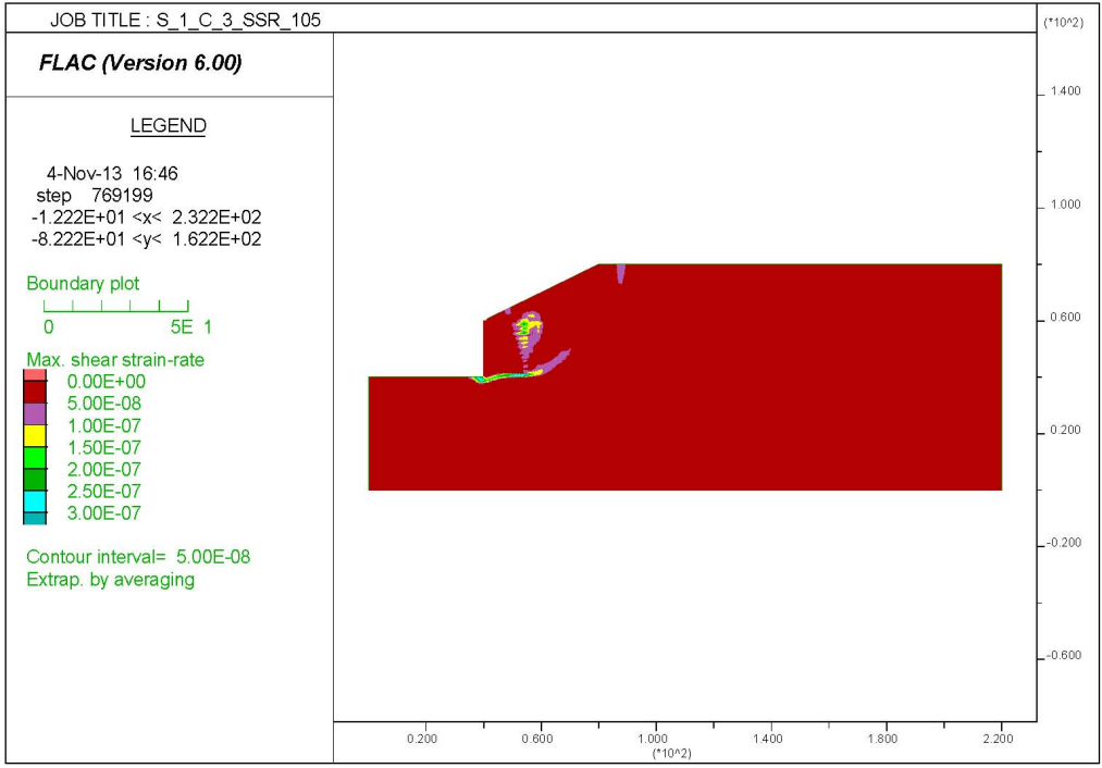
Figure C. 36. Series 1 Case 3 Foundation c_u=2000 psf, Backfill Angle \phi=34^\circ , and \gamma=105 pcf Maximum Shear Strain Rate.
