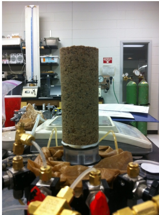
Figure 49. Sample Placed on the Bottom Cap of Triaxial Chamber.
