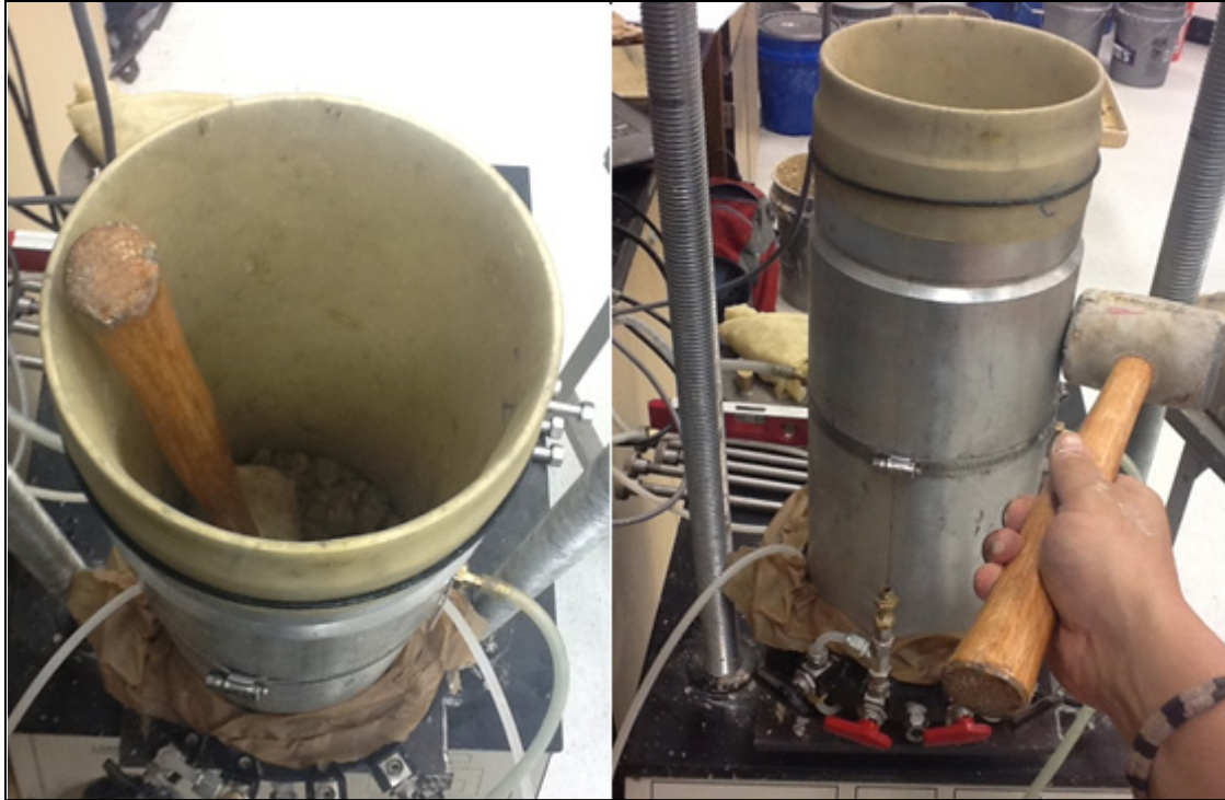
Figure 47. Compaction of Specimen.
