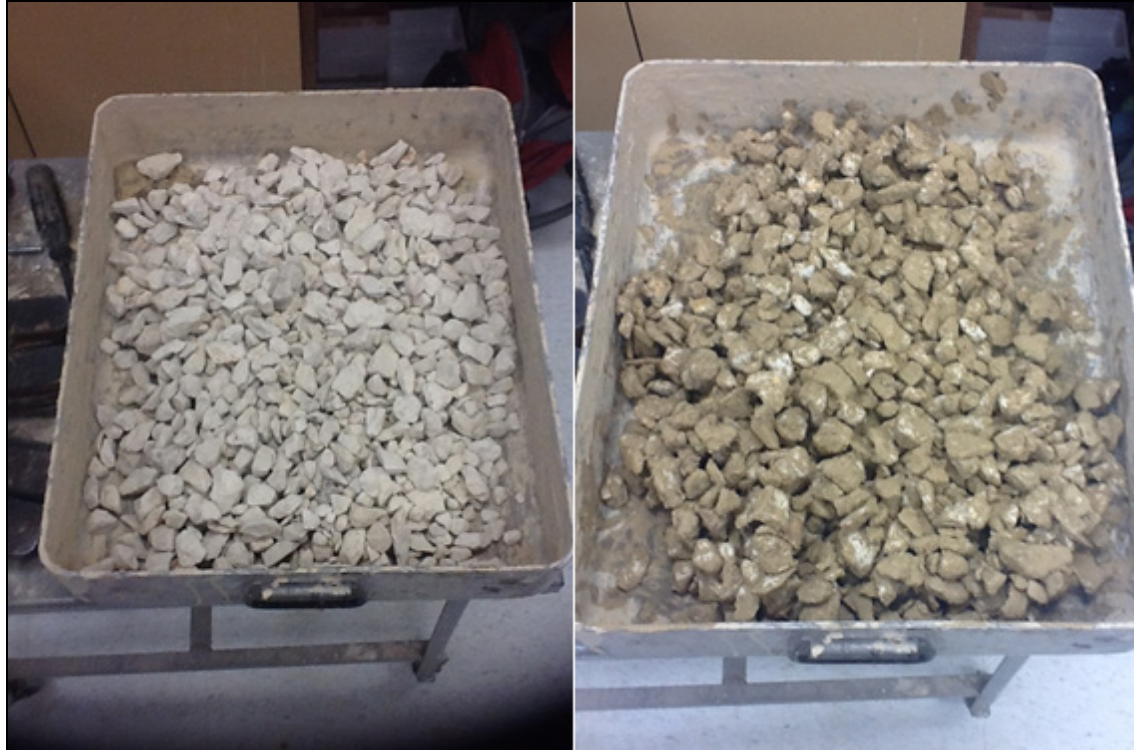
Figure 46. Sample Mixing of Passing #200 for Type D Material.
