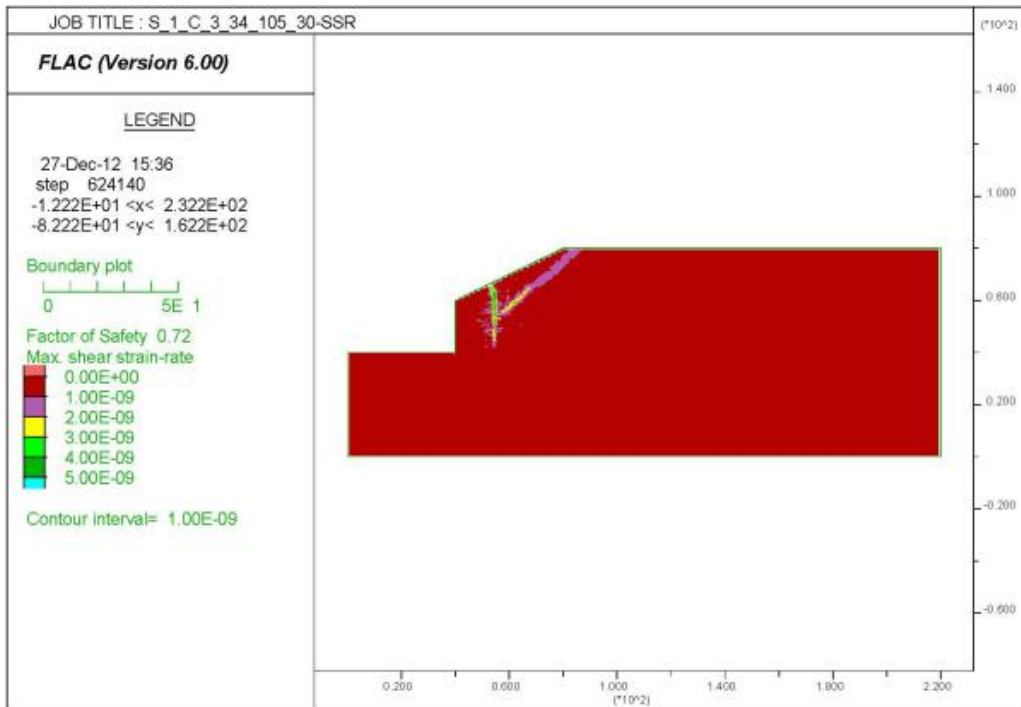
Figure C. 29. Series 1 Case 3 Foundation Angle \phi=30^\circ , Backfill Angle \phi=34^\circ , and \gamma=105 pcf Maximum Shear Strain Rate.
