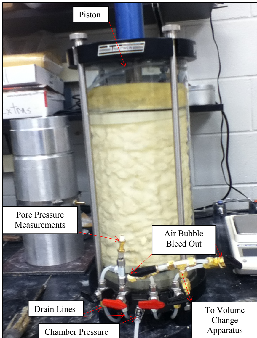
Figure 38. Large-Scale Triaxial Chamber.
