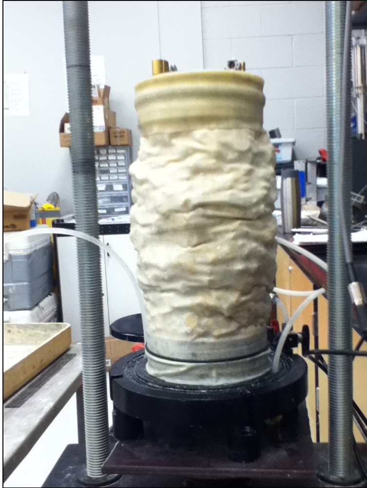
Figure 54. Parabolic Deformation of Test Specimen.
