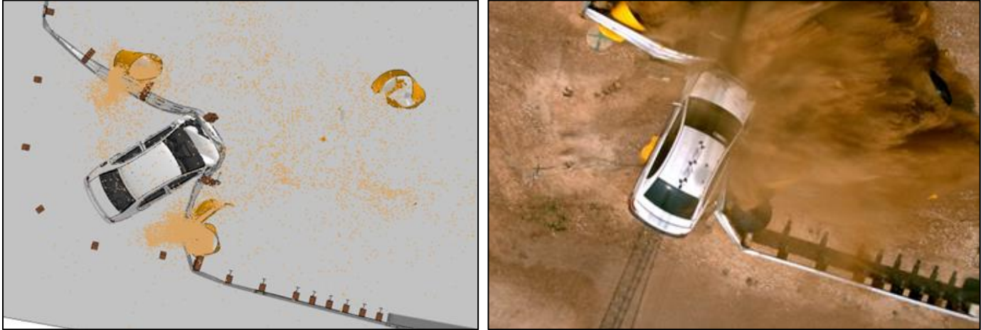
Figure 2. Simulation and Crash-Test Results with a Small Car.
