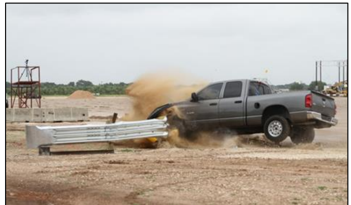
Figure 1. Simulation and Crash-Test Results with a Pickup Truck.
