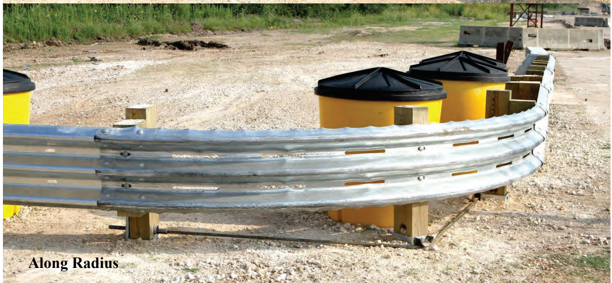
Figure 5.3. Short Radius Guardrail (Overall, Secondary Road, and Radius) prior to Test Nos. 467114-3 through 467114-6.
