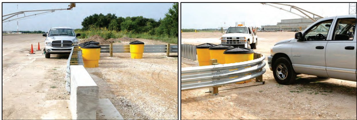
Figure 7.13. Vehicle/Installation Geometrics before Test No. 467114-5.
