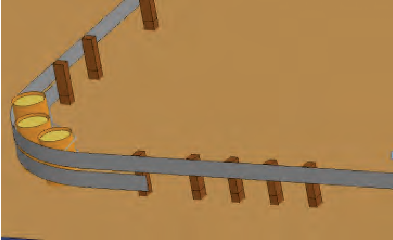
Figure 2.18. Short Radius Design of 3-Barrel System with Stacked Rail.
