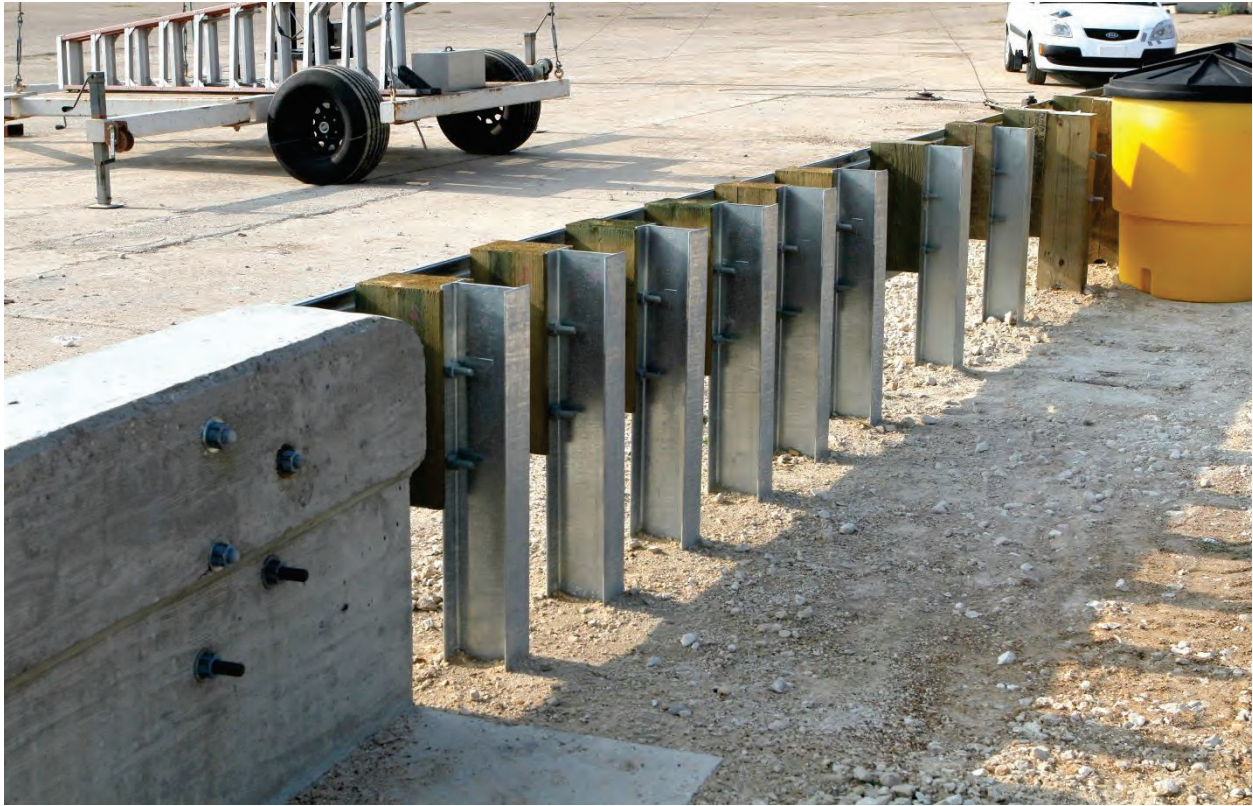
Figure 5.4. Short Radius Guardrail (Primary Road) before Test Nos. 467114-3 through 467114-6.
