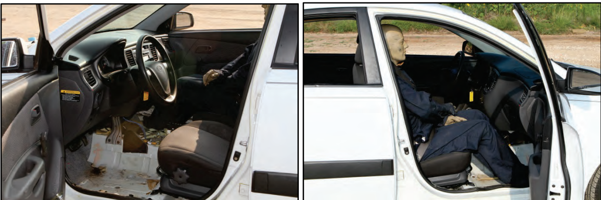
Figure 7.11. Interior of Vehicle after Test No. 467114-4.
