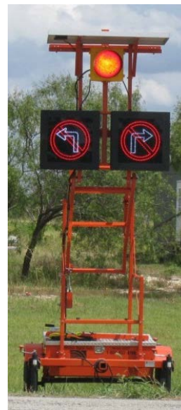
(a) Stop—No Turns Allowed.
