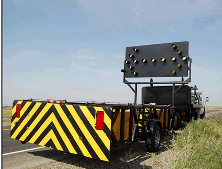
Figure 9. Energy Absorption’s Safe-Stop Trailer-Mounted Attenuator (36).
