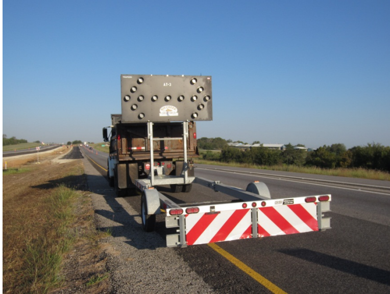
Figure 10. Gregory Industries' TTMA-100 Trailer-Mounted Attenuator.
