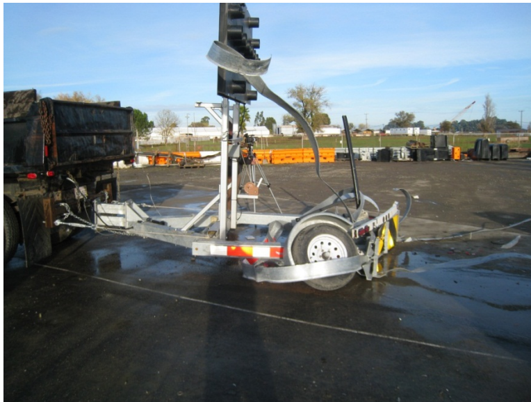
Figure 24. Post-Impact View of Arrow Panel on the TTMA-100 Trailer-Mounted Attenuator.
