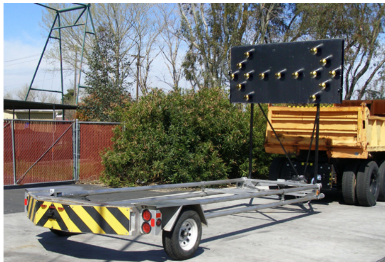
Figure 12. Energy Absorption’s Vorteq Trailer-Mounted Attenuator (45).
