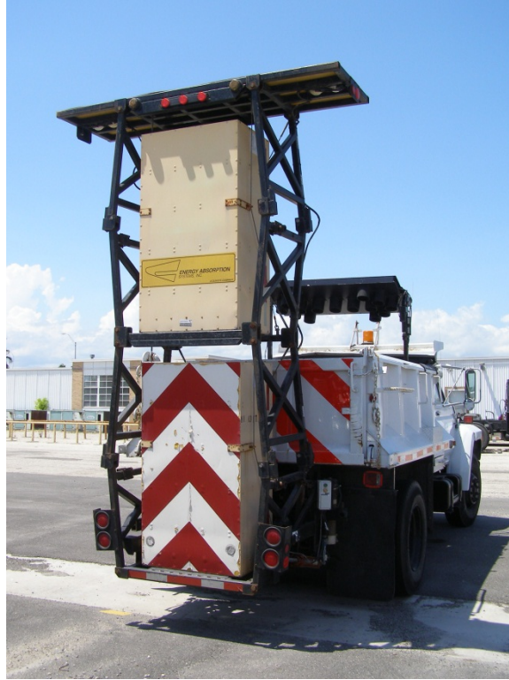
Figure 13. Safe-Stop 90 in Upright Position for Transport.
