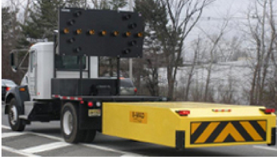
Figure 4. Barrier Systems' U-MAD Truck-Mounted Attenuator (26).
