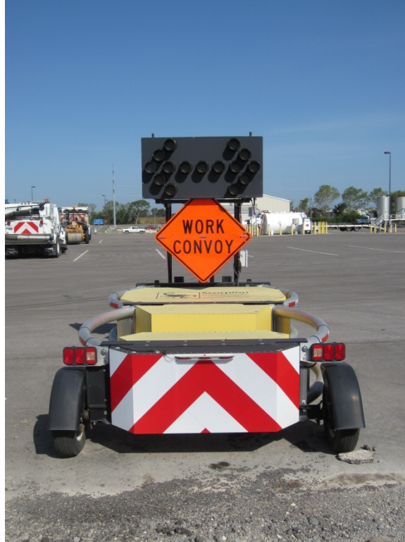
Figure 8. Traffix Devices' Scorpion Trailer-Mounted Attenuator.
