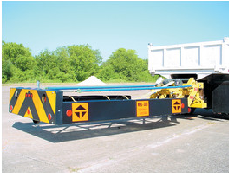
Figure 2. Trinity Industry's MPS 350 Truck-Mounted Attenuator (15).
