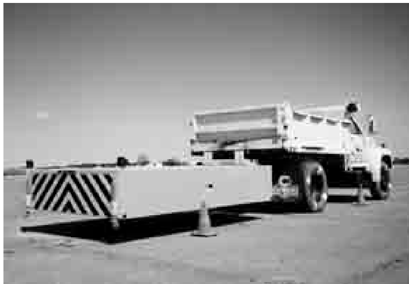
Figure 6. Renco's Ram 100K Truck-Mounted Attenuator ( 30 ).
