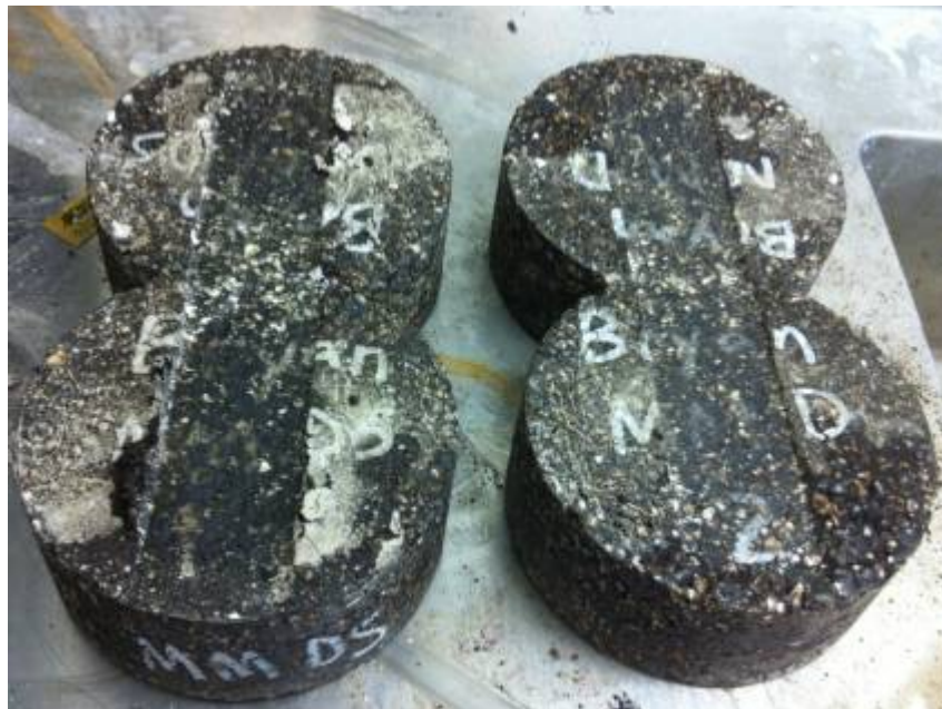
Figure 4.19. LRA Specimens after 20,000 Passes in a Dry Condition in the Hamburg Wheel Tracking Test.
