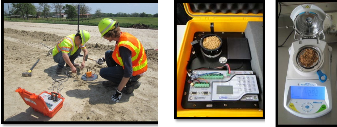
Figure 1. EDG, DOT 600, and Moisture Analyzer Tests.
