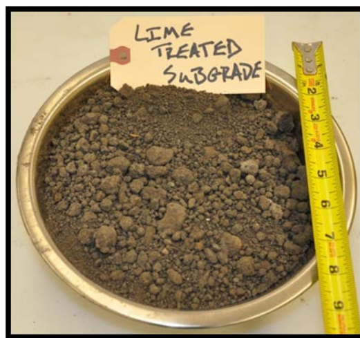
Figure 2.19. Representative LTS for Pilot Tests.
