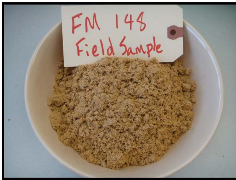
Figure 2.1. Low PI Soil Used in Pilot Tests with DOT 600 and Moisture Analyzer.
