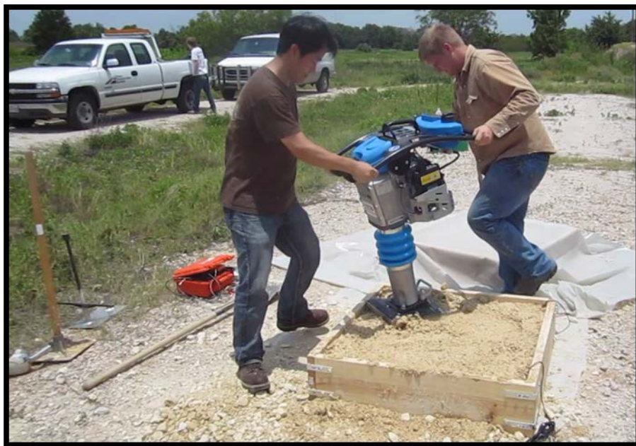
Figure 3.2. Mechanical Compaction of Test Box.
