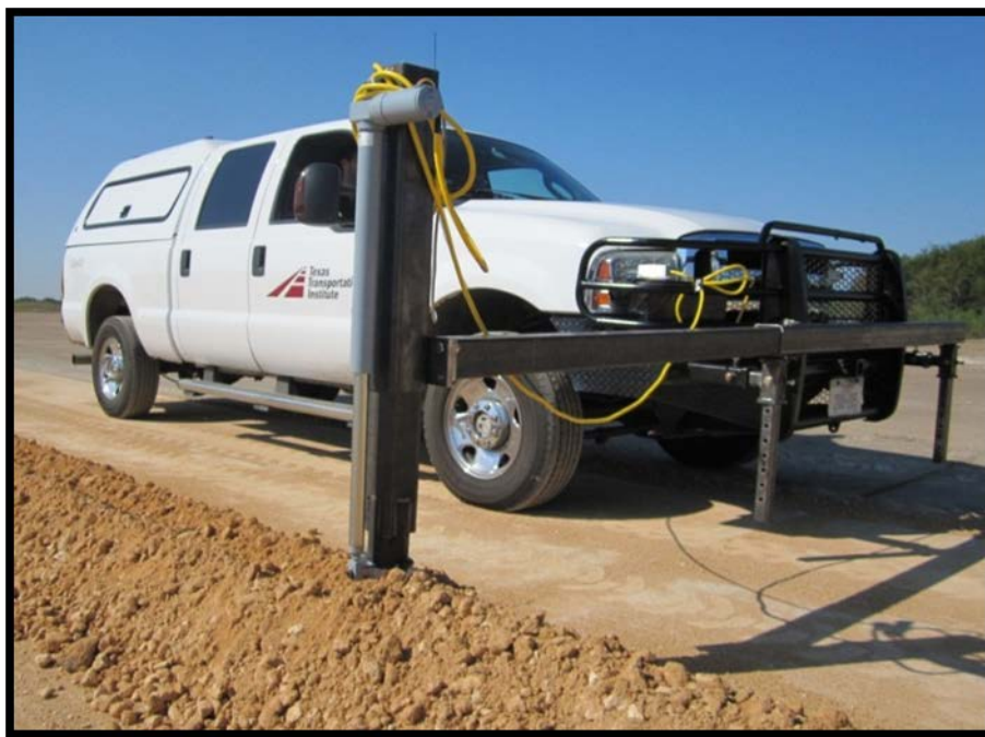
Figure 4.2. Measuring Windrow Moisture Content with Microwave Probe.
