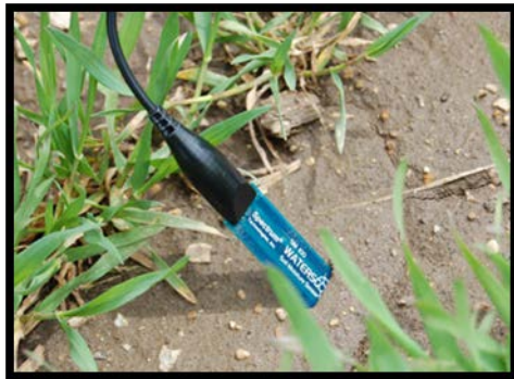
(a) WaterScout SM100 Sensor
