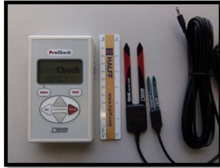
Figure 2.16. FDR Equipment for Pilot Testing with Flexible Base.
