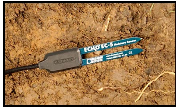
(b) Decagon EC-5 Moisture Sensor
