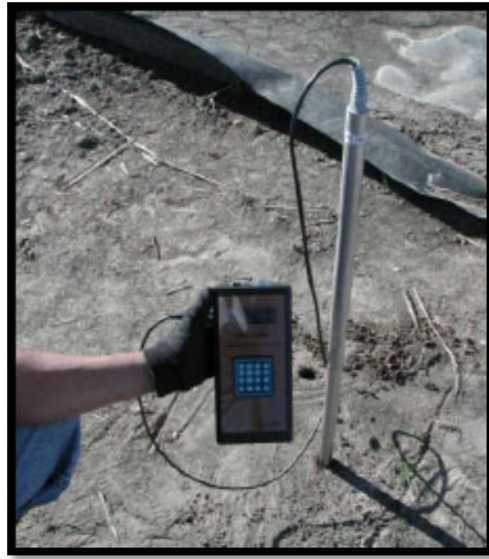
(b) Adek Down Hole Dielectric Probe
