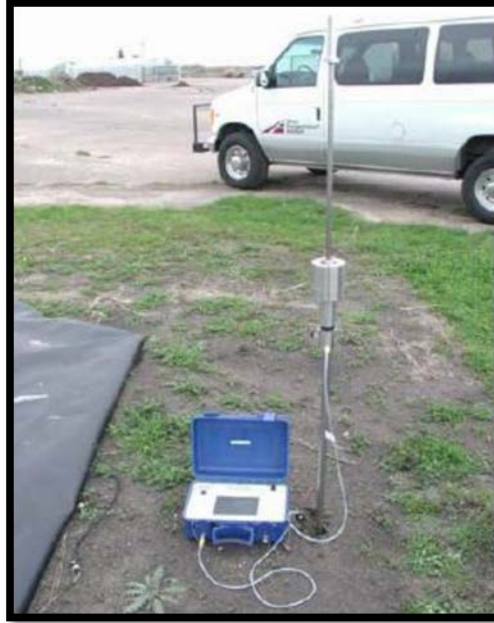
Figure 1.11. Vertek SMR Probe.
