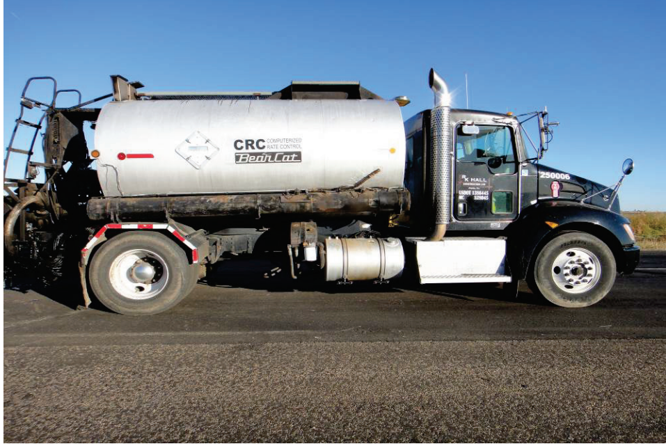
a. Tack Coat Spraying Machine.
