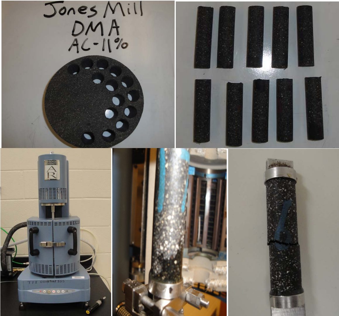
Figure 19. DMA Specimen Preparation and Test Setup.
