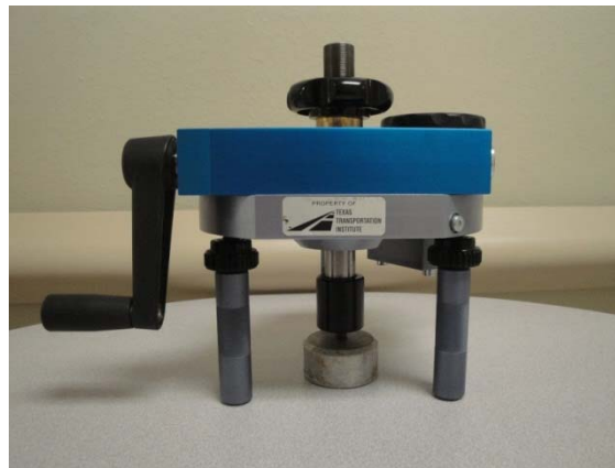
Figure 13. Photo of Direct Tensile Bond Test Apparatus.
