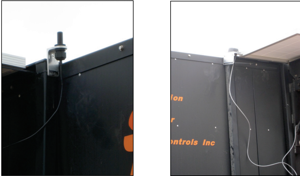
Figure 2. Temporary Attachments of GPS and Satellite Communication Antennae to a Precision Solar Controls PCMS.
