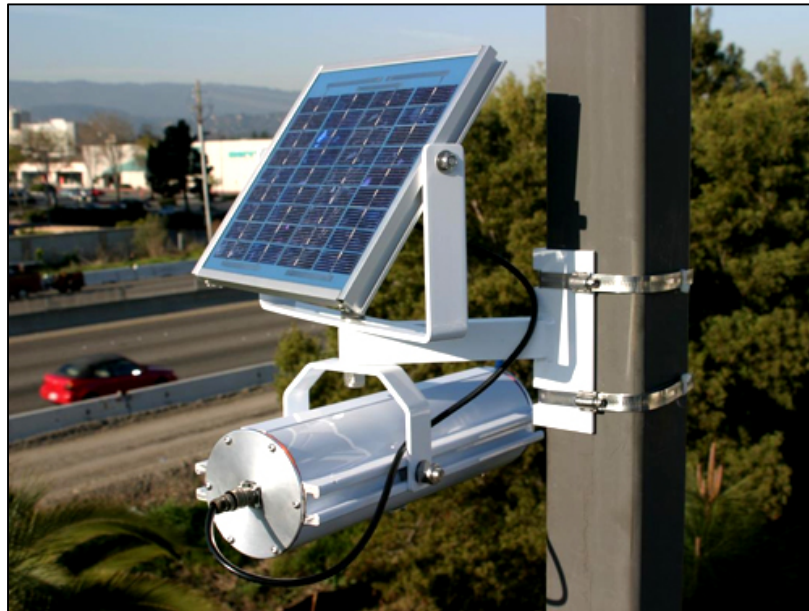
Figure 10. SpeedInfo Doppler Radar Sensor.
