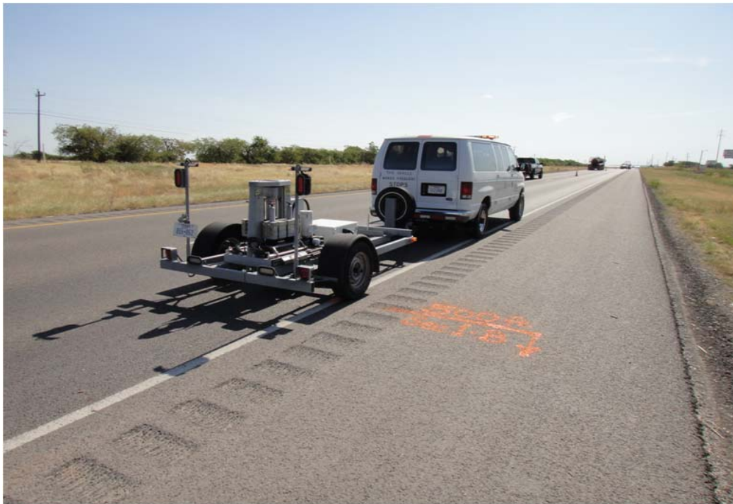
Figure 6-5. Example FWD Testing on SH 114 (Fort Worth, Summer 2011).
