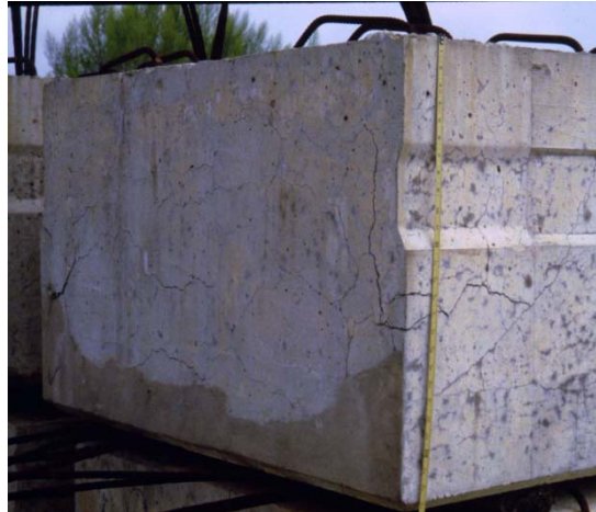
Figure 2.2. Prestressed Concrete Box Beams Cast in 1991 Started Showing Cracking in 1993 while Still in Storage.
