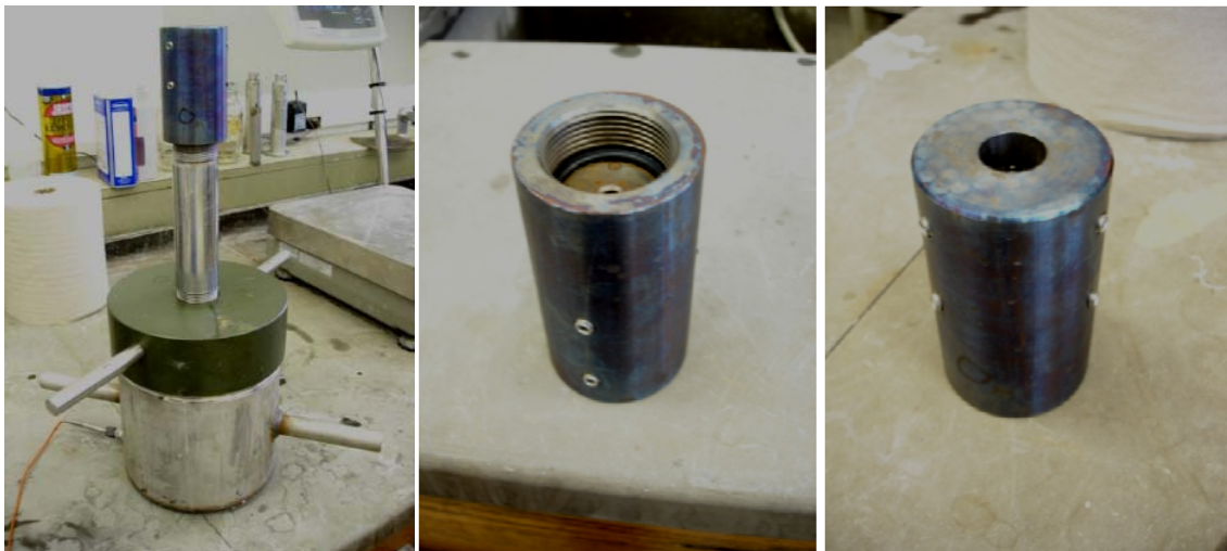
Figure 4.3. A Modified VCMD with LVDT Housing.
