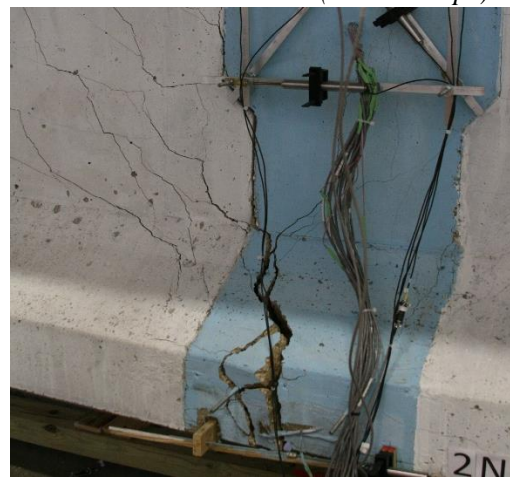
(c) Splice 2 - South View, Shear Slip after the Crack Widened ( P = 334 kips)
