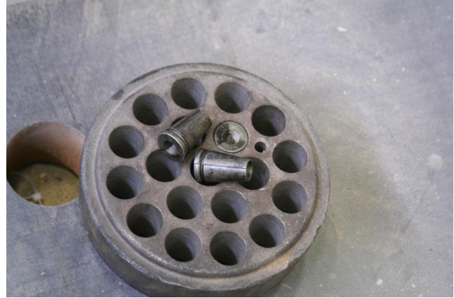
(b) Anchorage Plate and Anchor Wedges
