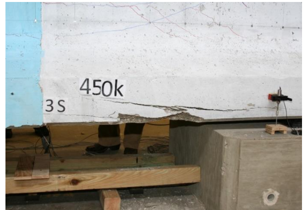
(e) Compression Failure ( P = 450 kips)
