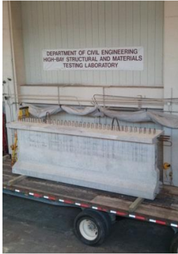
(a) Girder Segments with Lifting Points
