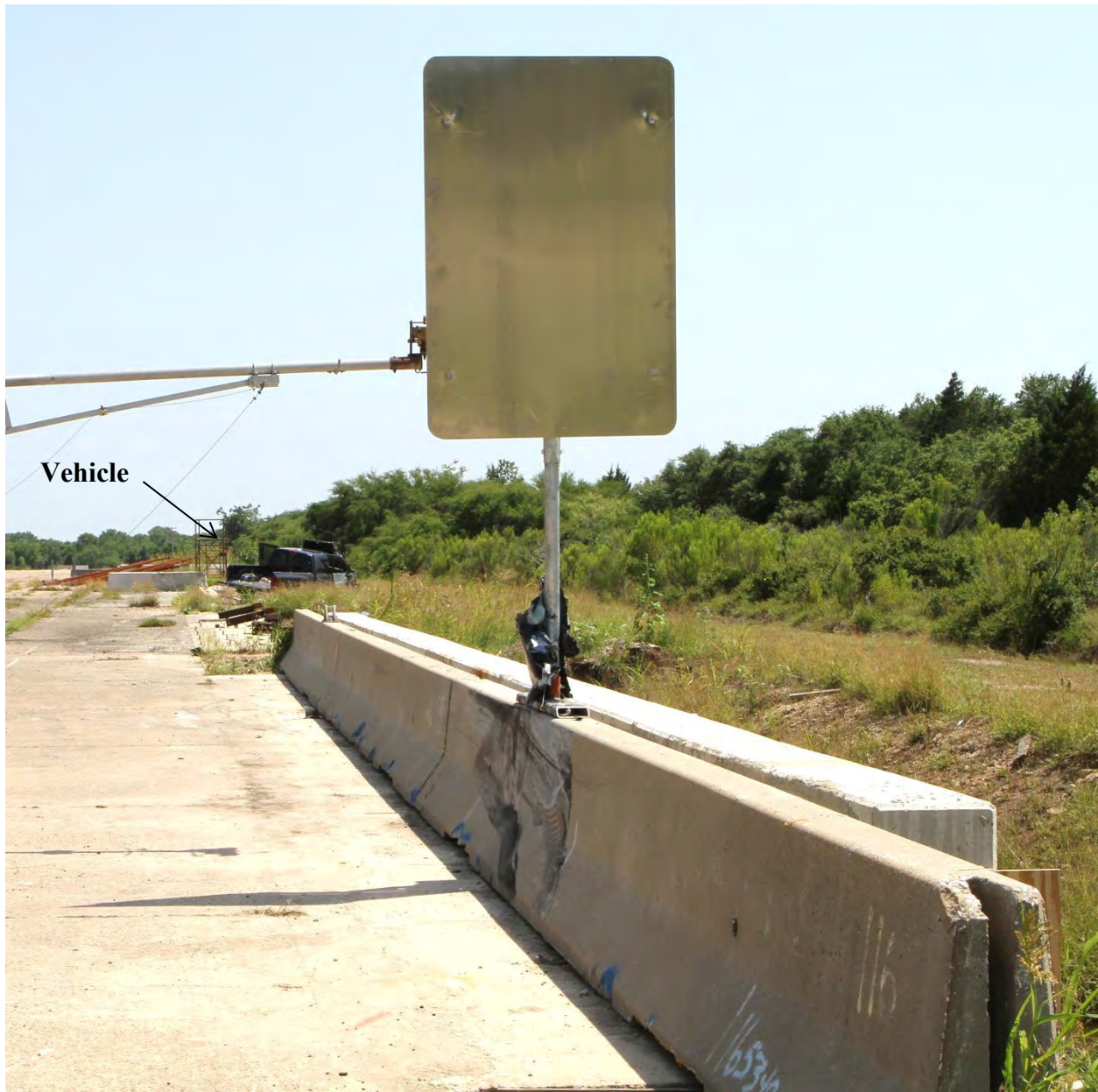
Figure 6.8. Vehicle/Spread Tube Sign Support System on CMB Positions after Test No. 466462-1.
