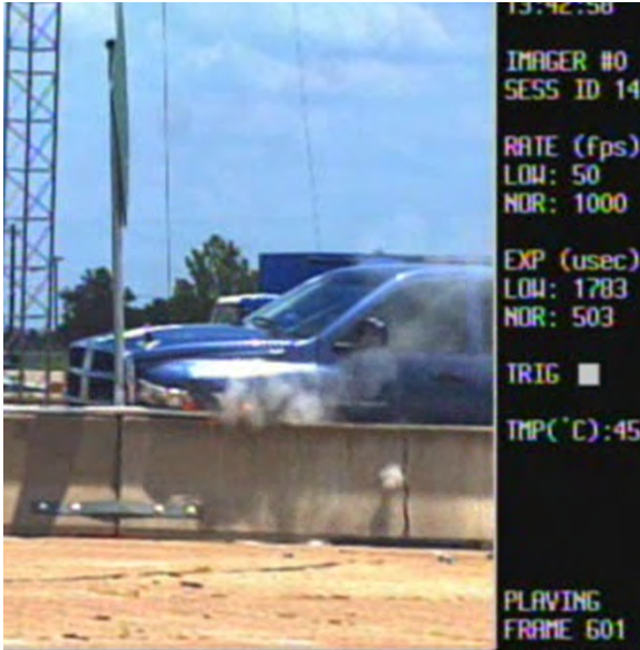
Video 1C (Frame 601) Vehicle Impacts the pole in Frame 601. t=(601-520)/1000=0.081 s
