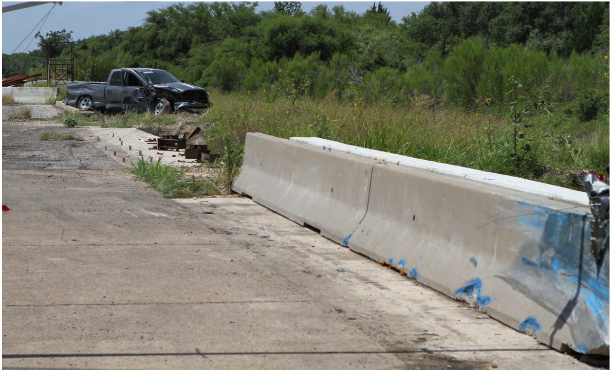
Figure 6.17. Vehicle/Bracket and Sacrificial Pin Sign Support on CMB after Test No. 466462-2a.
