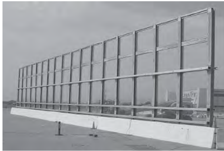
Figure 2.12. Noise Wall Barrier System Used in MwRSF Test (13).
