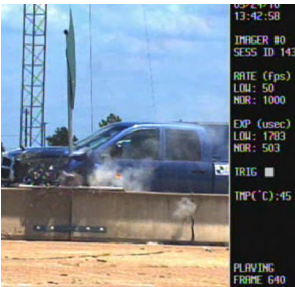
Video 1C (Frame 640) Vehicle fender snags into the pole in Frame 641. t=(640-520)/1000=0.121 s
