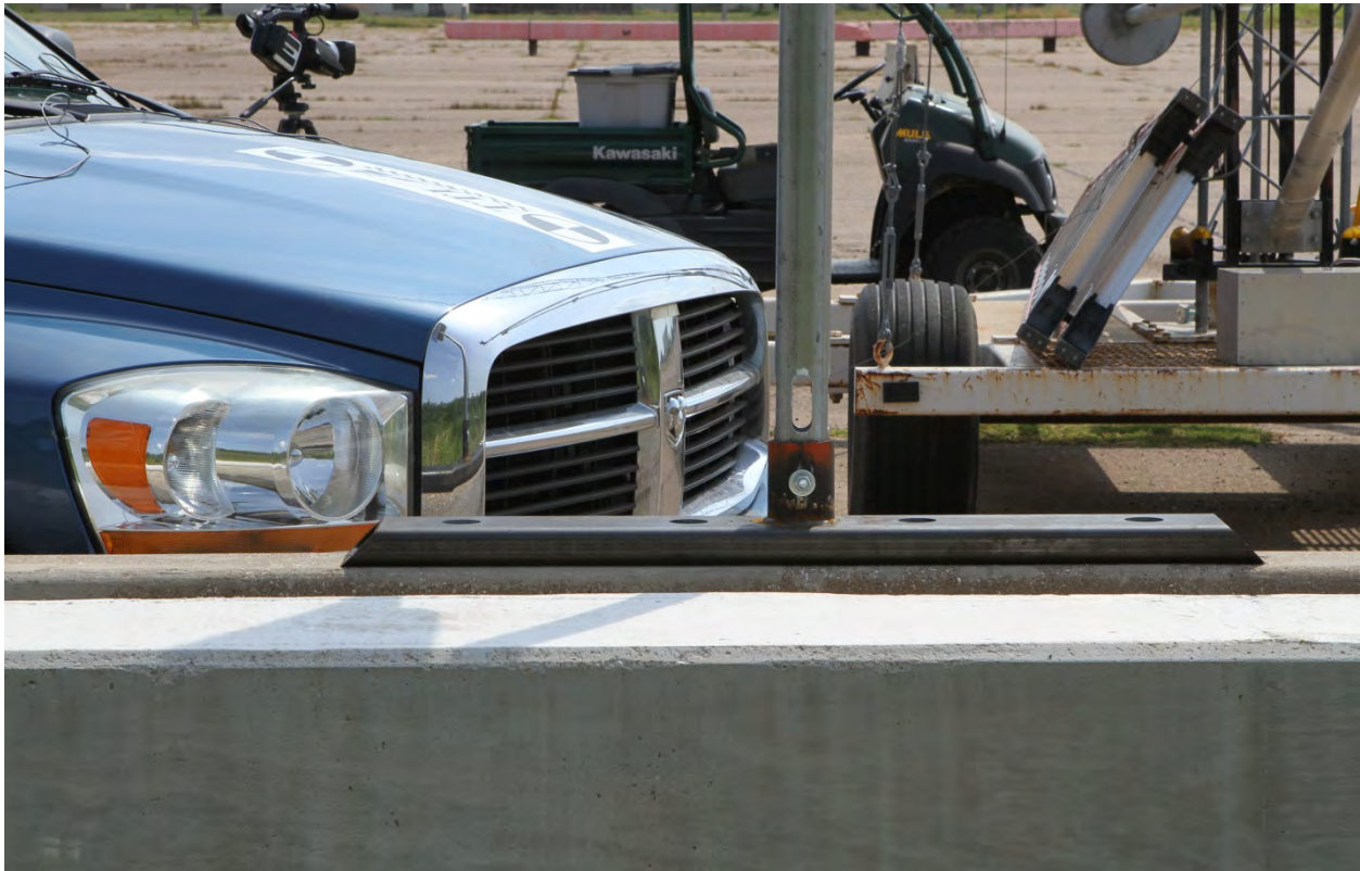
Figure 6.33. Vehicle/Slotted 10 BWG Sign Support on CMB Geometrics for Test No. 466462-4.
