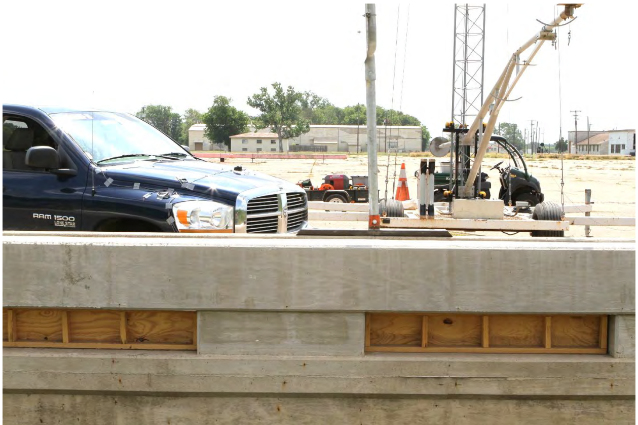
Figure 6.6. Vehicle/Spread Tube Sign Support System on CMB Geometrics for Test No. 466462-1.
