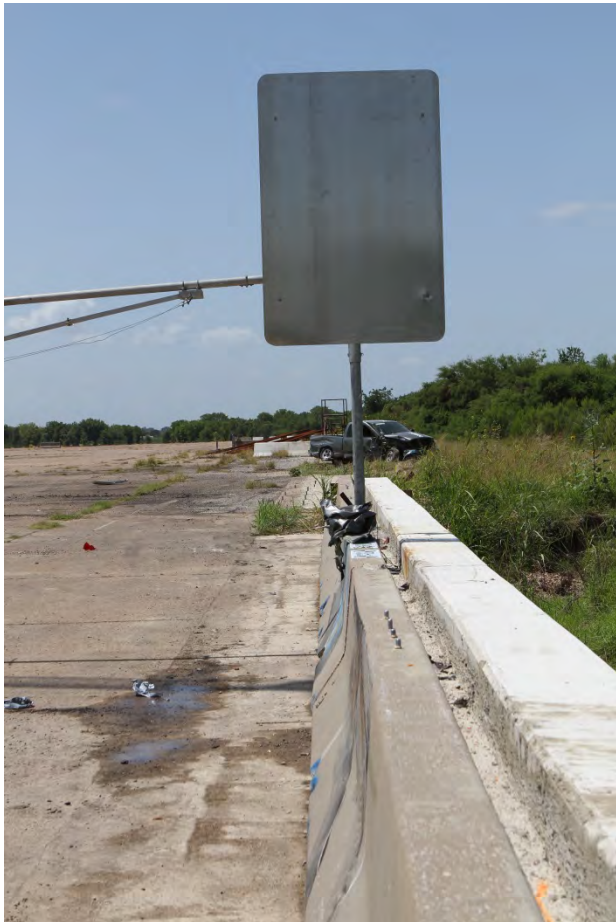
Figure 6.18. Bracket and Sacrificial Pin Sign Support on CMB after Test No. 466462-2a.
