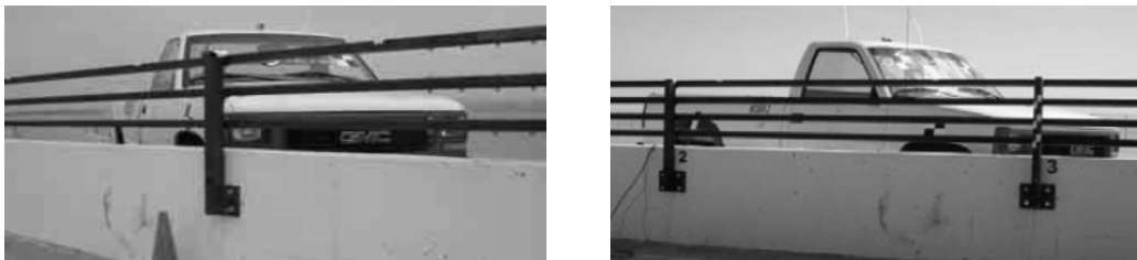
Figure 2.14. Setup for Crash Tests (MOBR1 and MOBR2) Performed on Two Combination Traffic/Bicycle Bridge Railing Systems Designed at MwRSF (14).
