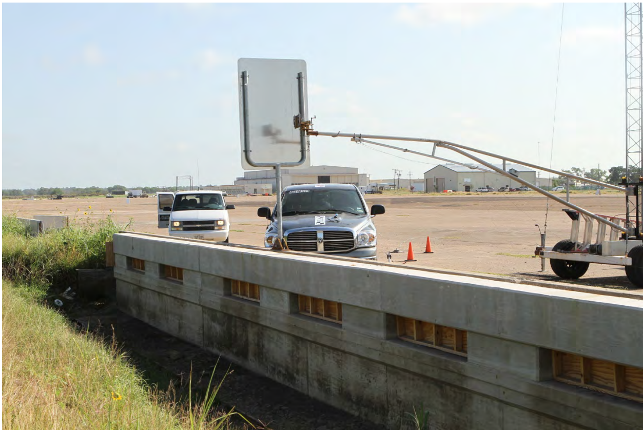
Figure 6.15. Vehicle/Bracket and Sacrificial Pin Sign Support on CMB Geometrics for Test No. 466462-2a.
