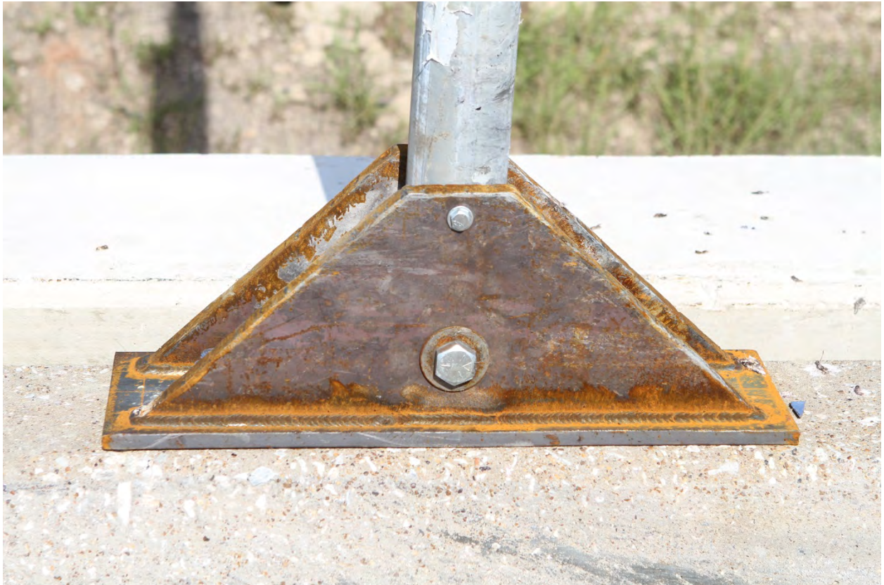
Figure 6.14. Bracket and Sacrificial Pin Sign Support on CMB before Test No. 466462-2a.
