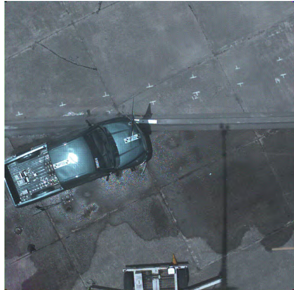
Video 1C (Frame 601) Vehicle Impacts the pole in Frame 601. t=(601-520)/1000=0.081 s
