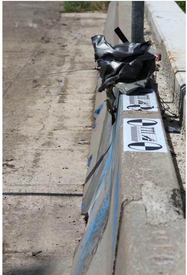
Figure 6.18. Bracket and Sacrificial Pin Sign Support on CMB after Test No. 466462-2a.
