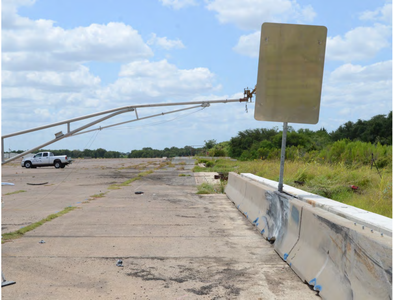
Figure 6.26. Vehicle/Chute Channel Sign Support on CMB after Test No. 466462-3.
