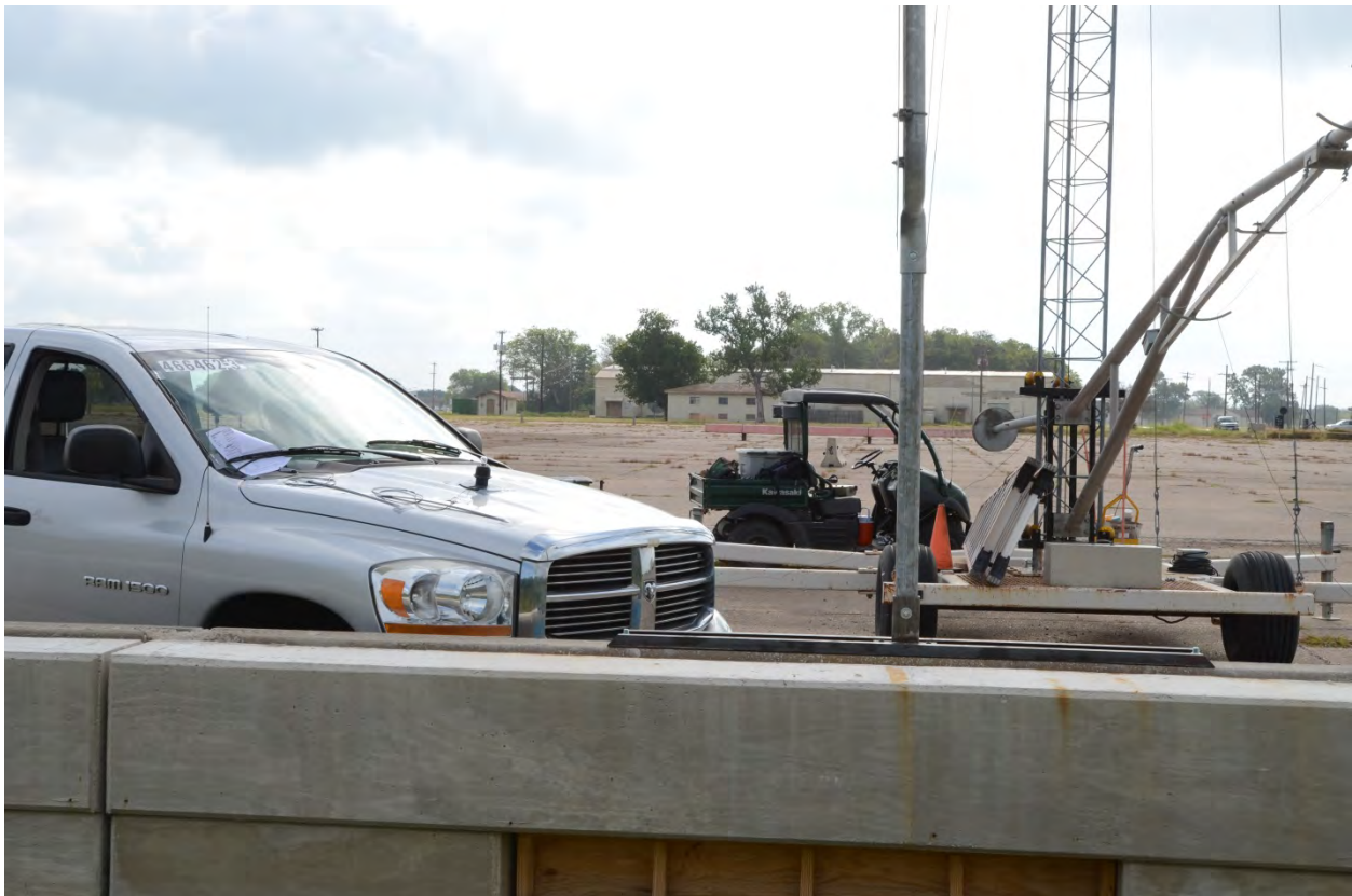
Figure 6.24. Vehicle/Chute Channel Sign Support on CMB Geometrics for Test No. 466462-3.
