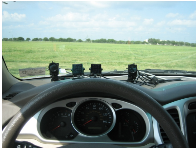
Figure 4. Eye Tracking System on the TTI Instrumented Vehicle's Dash.
