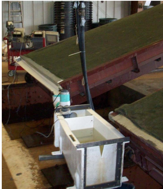
Figure 4. Erosion Control Performance Tests Using Coagulants.
