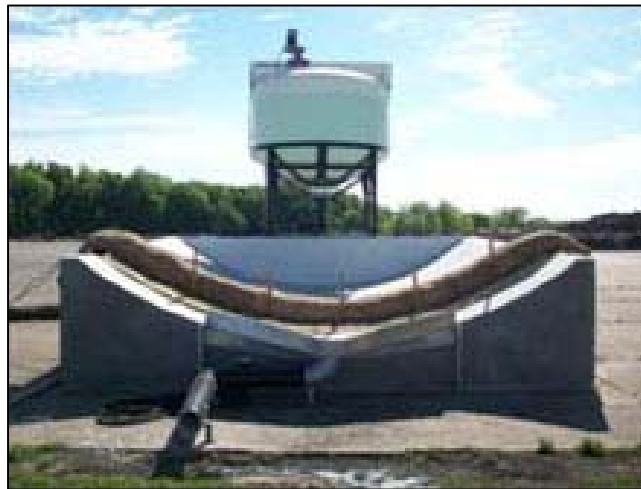
Figure 5. Sediment Retention Device Testing Flume.
