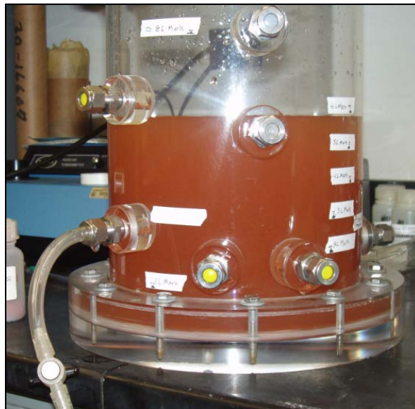
Figure 7. Decanter Used to Remove Large Particles from Soil Suspension.
