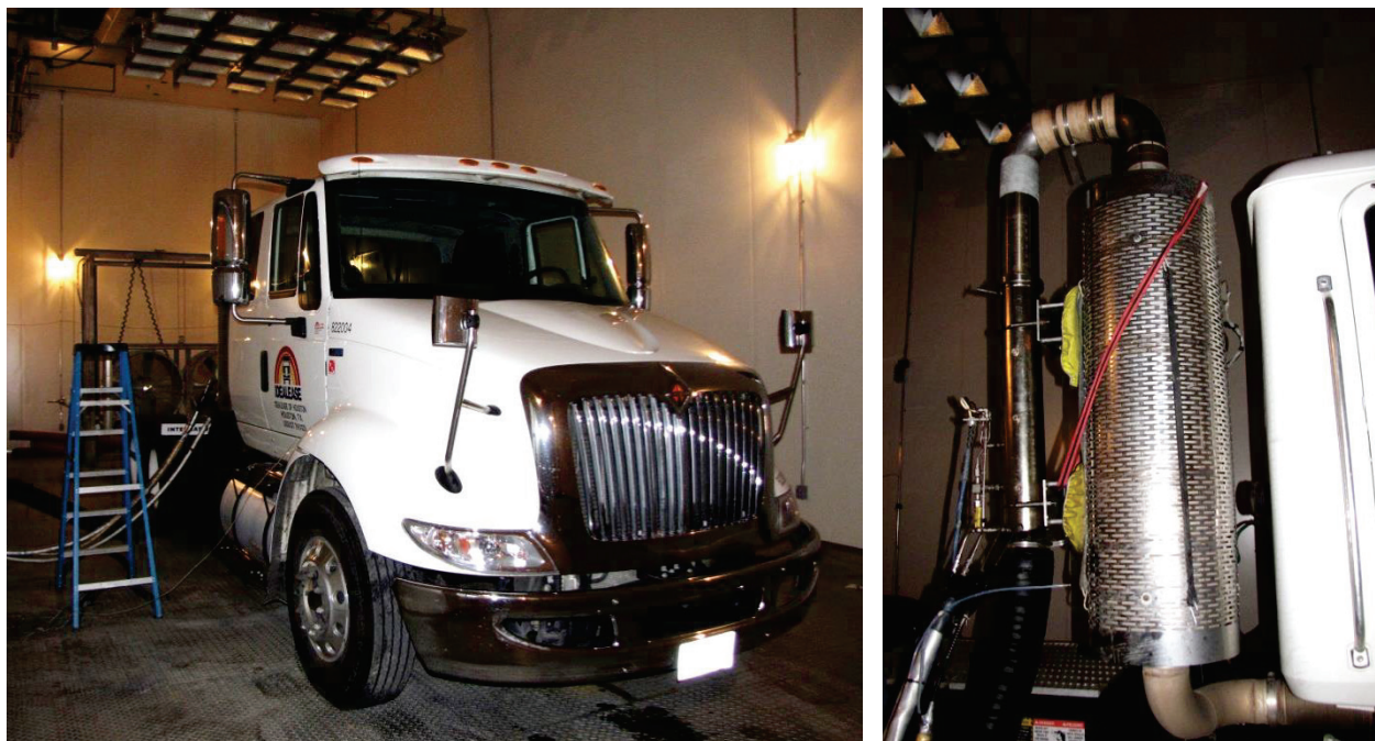
Figure 16. Test Vehicle (Left) and Sampling Lines Installed on a Test Vehicle (Right).
