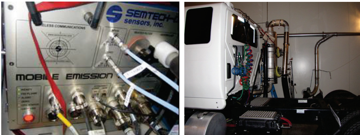
Figure 18. SEMTECH-DS (Left) and EFM Installed on a Test Truck (Right).
