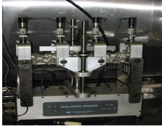
Figure 2-9. Beam Fatigue Apparatus and Specimen (after Prowell et al. 2010).
