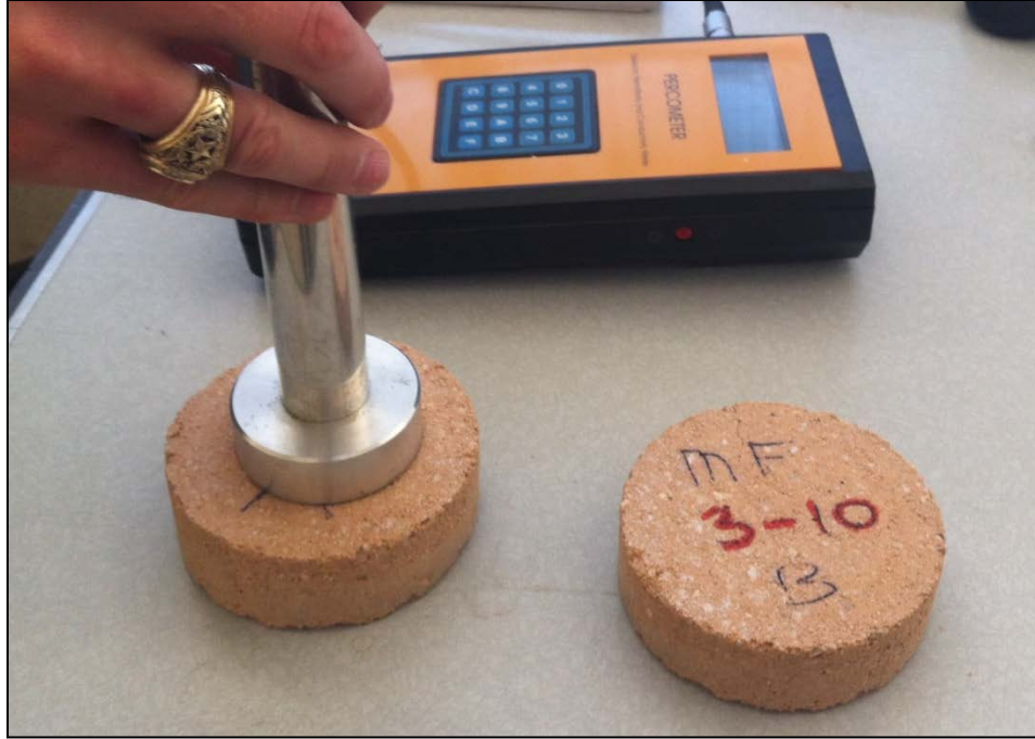
Figure 6.23. A Percometer Reads the Dielectric Constant of Compacted Soil Samples.
