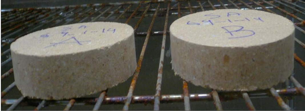
Figure 6.45. Two Compacted Soil Samples Are Placed in an Environment Room.
