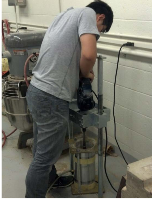
Figure 6.3. Process of Vibratory Compaction.
