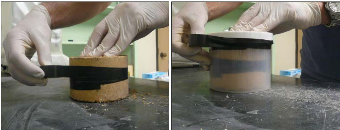
Figure 6.15. Filter Papers Are Placed in between and on Top of the Samples and Samples Are Sealed.
