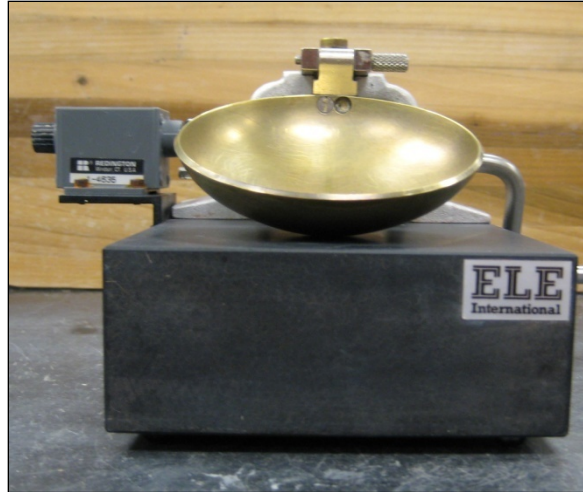
Figure A.3. Hand-Operated Liquid Limit Device.
