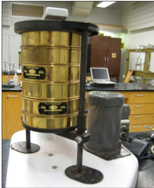
Figure A.1. Sieves and Sieve Shaker for Tex-110-E.
