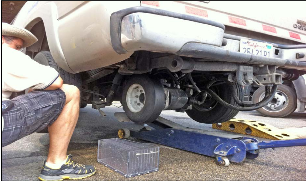
Figure 31. Dynatest 6875H Wheel Assembly with Test Tire.
