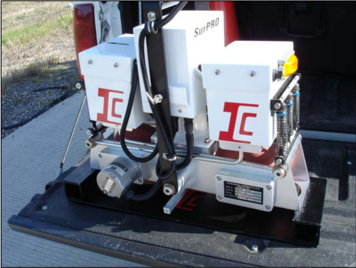
Figure 5. SurPRO Reference Profiler Used to Determine Grade Change Profile.
