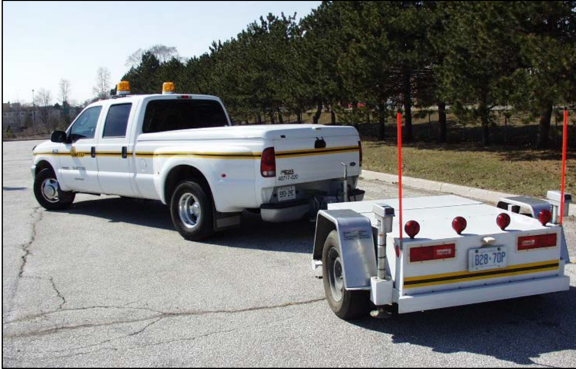
Figure 47. New ASTM E274 Skid Measurement System.
