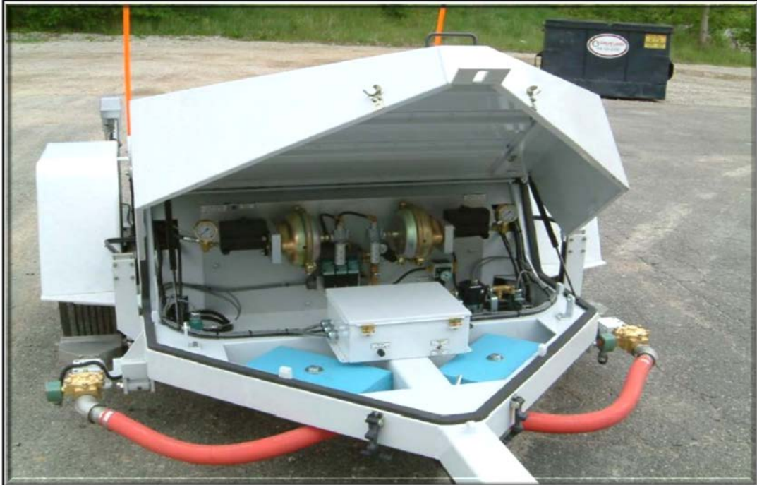
Figure 46. ICC ASTM E274 Trailer.
