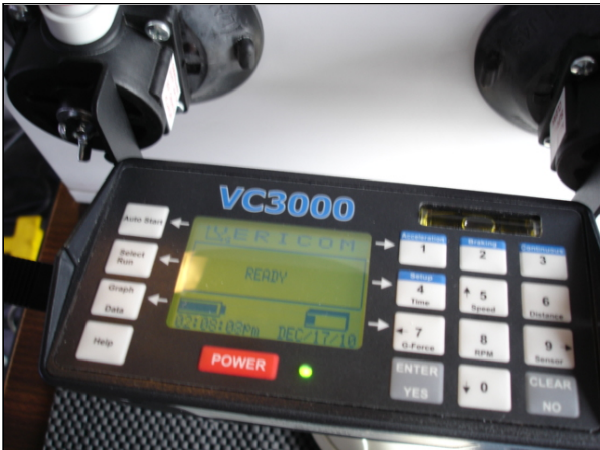
Figure 3. Instrument Used to Measure Vertical and Lateral Accelerations.
