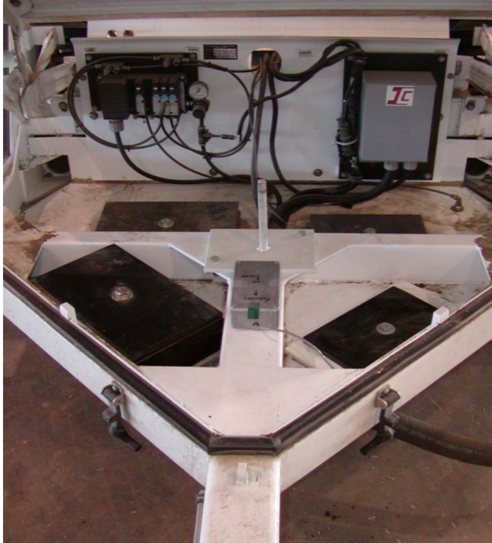
Figure 42. Accelerometer Unit Mounted on TTI E274 System.
