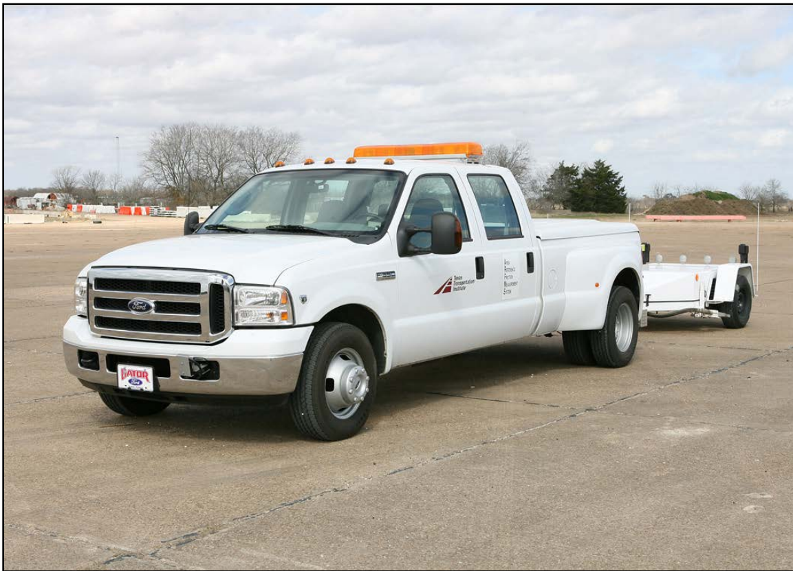
Figure 17. TTI E274 Friction Measurement System.
