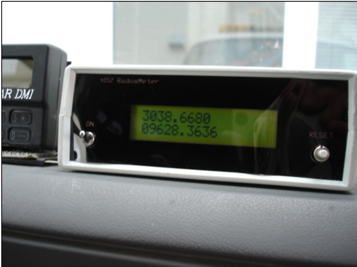
Figure 4. Photo of RadiusMeter for Measuring Radius of Curvature.
