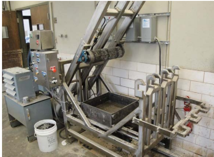
Figure 4.5. PMW Linear Compactor for Molding Slabs.
