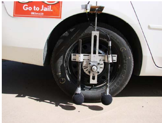
Figure 7.2. On-Board Sound Intensity System.
