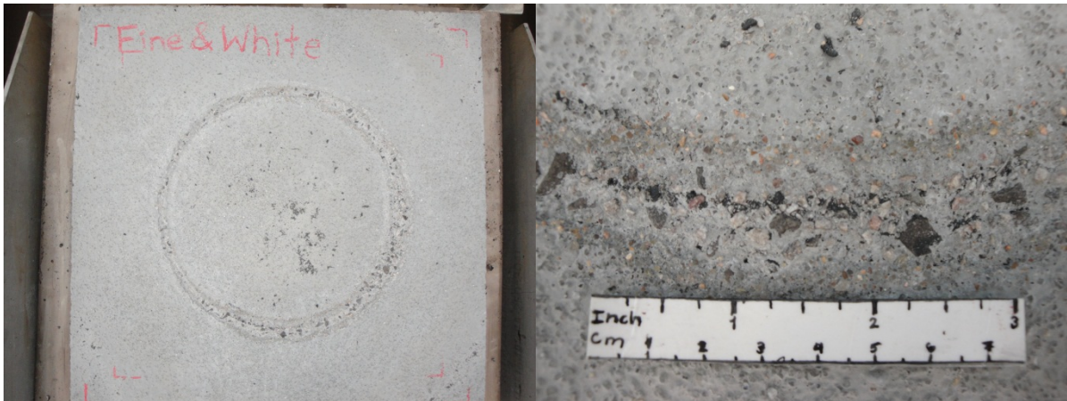
Figure C.12. Tuffseal (F+W) Slab (2,000 Cycles).
