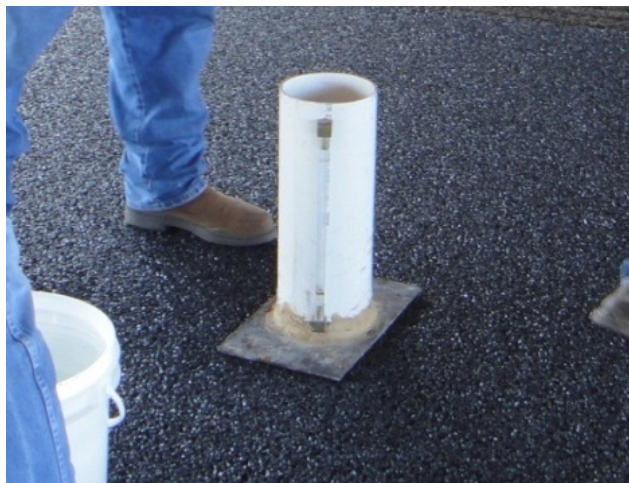
Figure 7.3. Water Flow Test.
