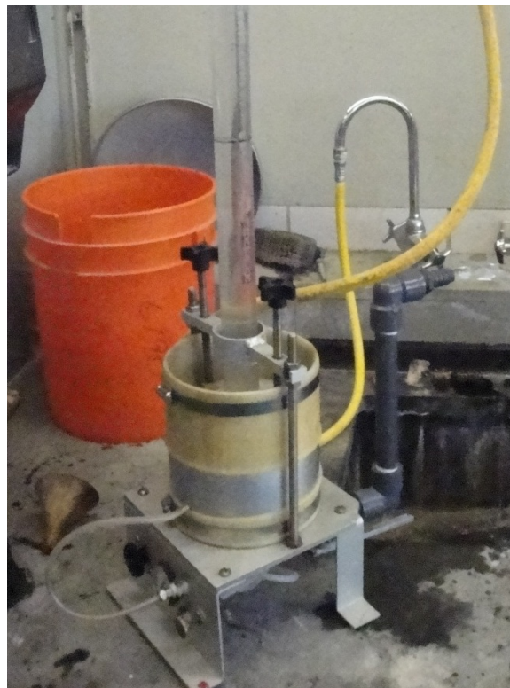
Figure 4.4. Florida Falling-Head Permeameter.
