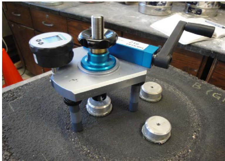
Figure 5.4. Pull-Off Test Device.
