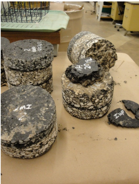
Figure B.24. Flushed and Moisture-Damaged Core Specimens (Atlanta-Fine SMA).
