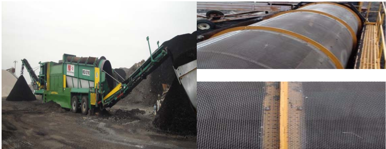
Figure 6. Screening RAS Using Trommel Screen Machine.
