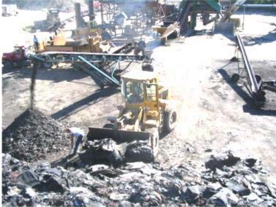
Figure A-2. Front-End Loader Moving Material from a Pile of Source Separated TOAS (after Krivit, 2007).
