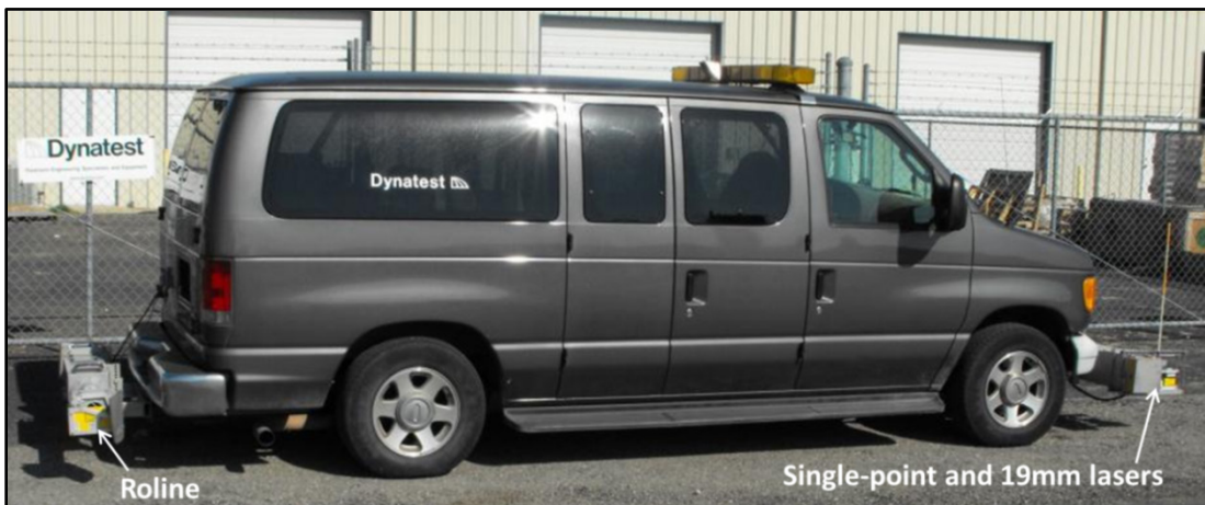
Figure 5.1. Dynatest Three-Laser System.
