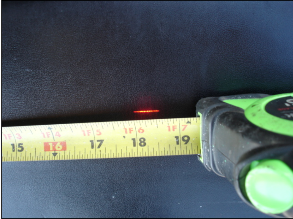
Figure 1.2. 19mm Wide-Spot Laser from LMI/Selcom.
