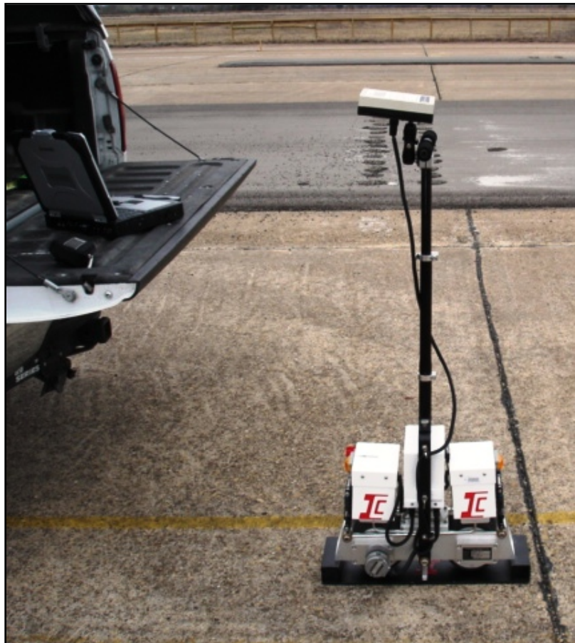
Figure 3.1. SurPRO 3500 Reference Profiler.
