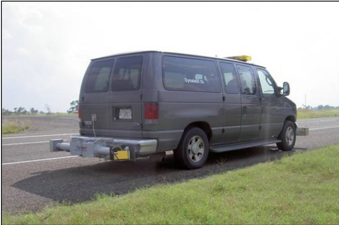
Figure 2.15. Dynatest Profiler Van Used in 2009 Comparative Laser Testing.
