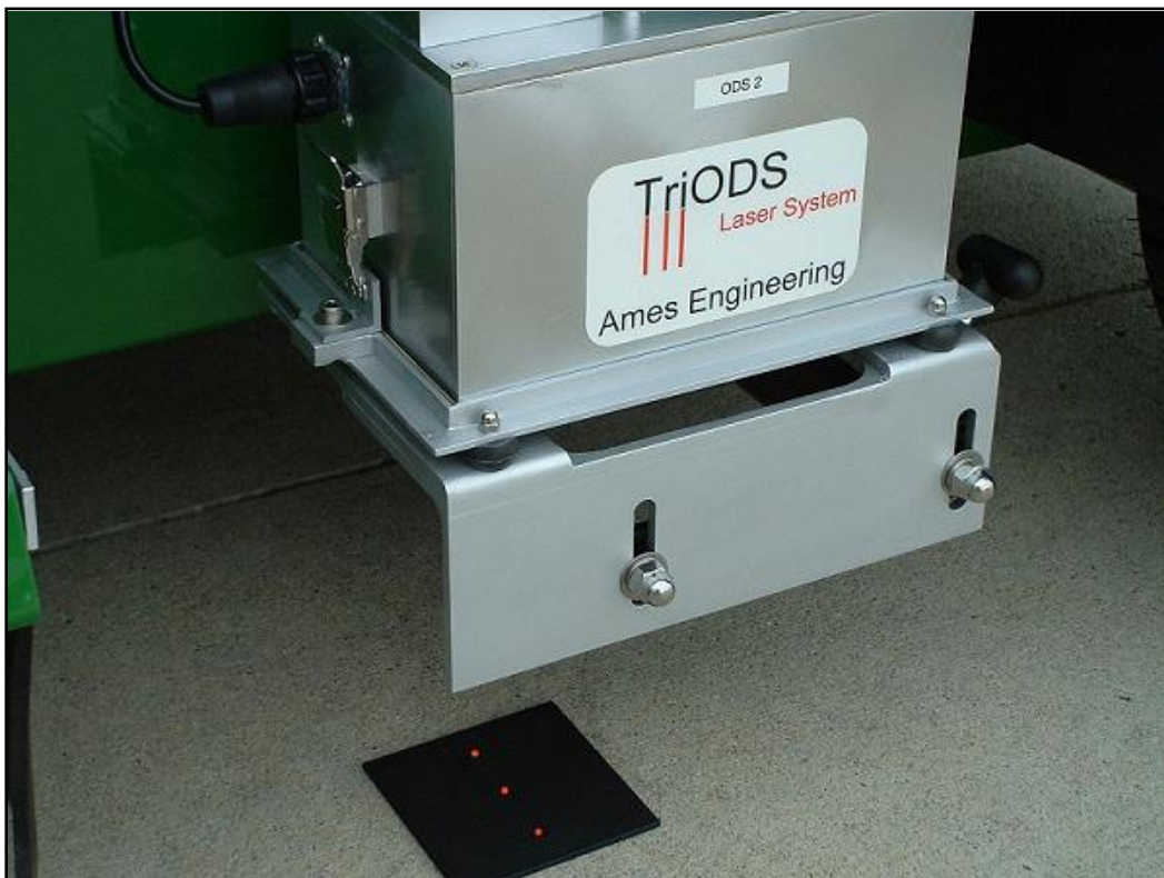
Figure 1.1. TriODS Three-Laser System from Ames Engineering.
