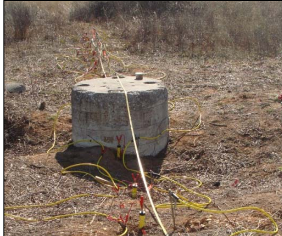
Figure 12-19. Deep Foundation with Optimal Electrode Placement.
