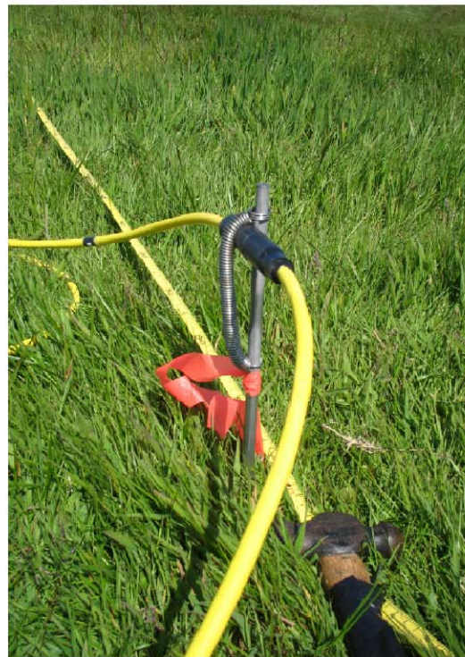
Figure 10-8. (Left) Multi-electrode Resistivity System from Advanced Geosciences, Inc.; (Right) Close-up of an Electrode Installation.
