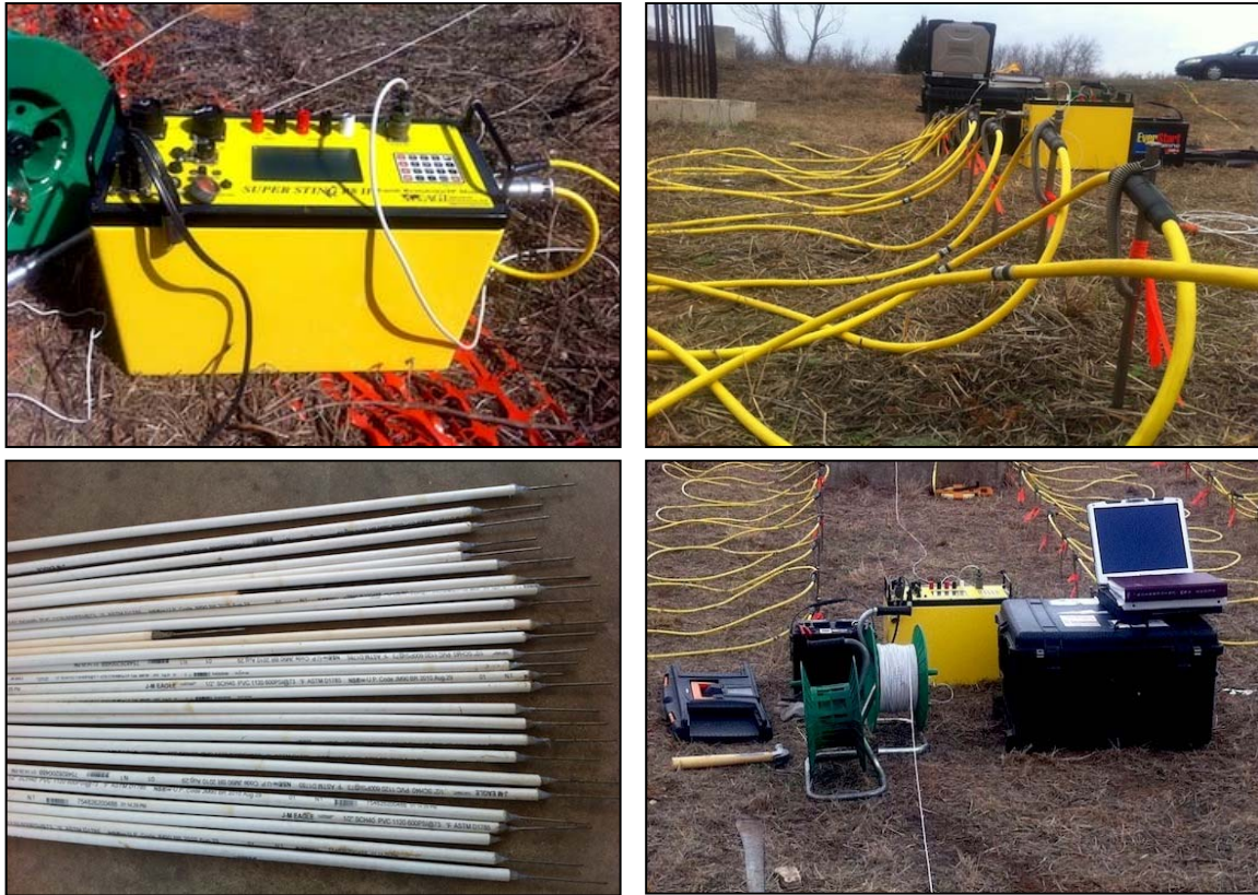
Figure 11-1. (Upper Left) AGI SuperSting™ R8/IP Meter; (Upper Right) Electrodes Connected to the Cable Takeouts; (Lower Left) Underwater Electrodes; (Lower Right) Field Setup.
