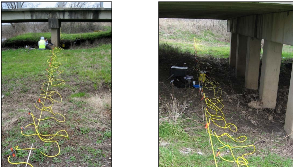
Figure 11-8. Bridge 15 ERI Fieldwork.
