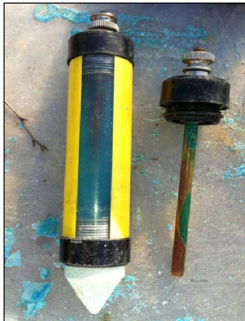
Figure 10-16. Non-polarizing Electrode and Copper Core.
