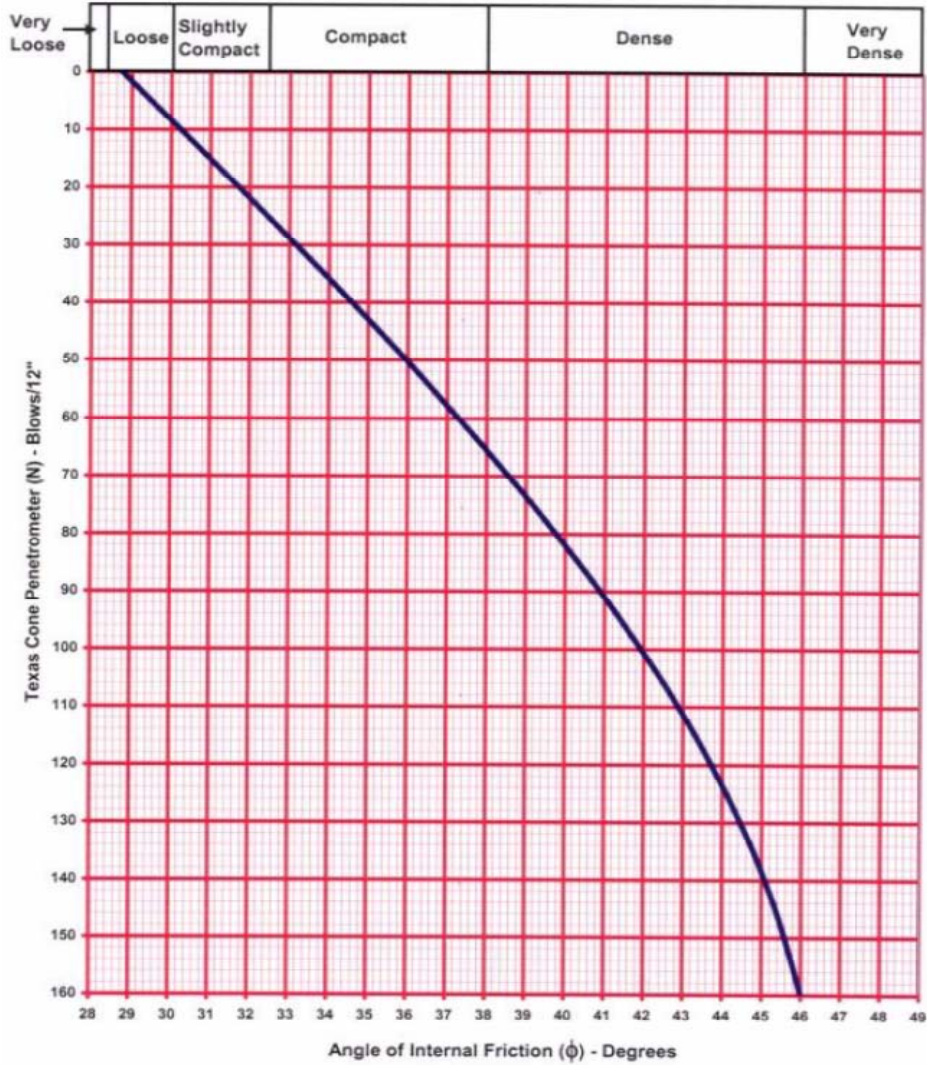
Figure 6-1. Angle of Friction for Cohesionless Soils.
