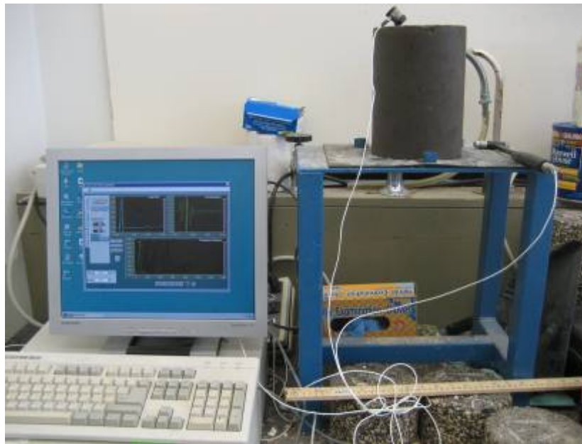
Figure 57. Free-Free Resonant Column Test.
