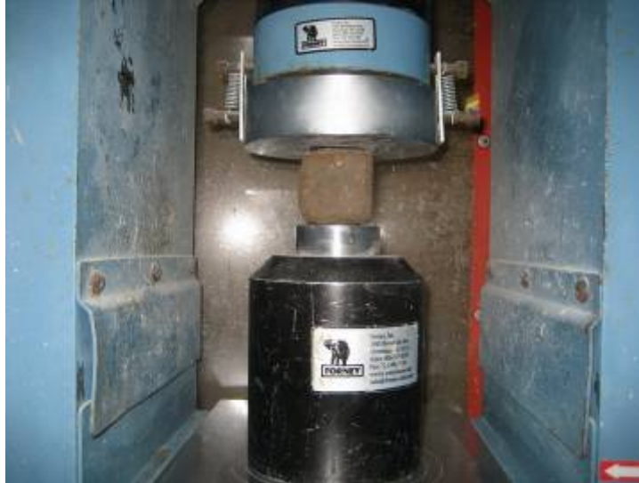
Figure 90. Compressive Strength Test.
