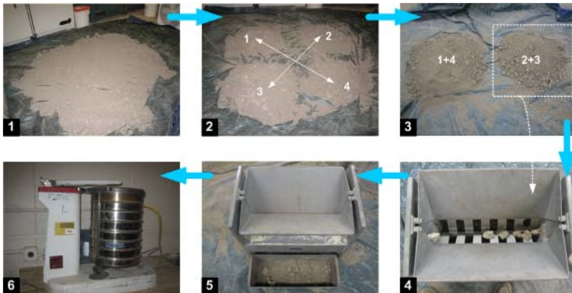
Figure 49. Particle Size Analysis Procedure.
