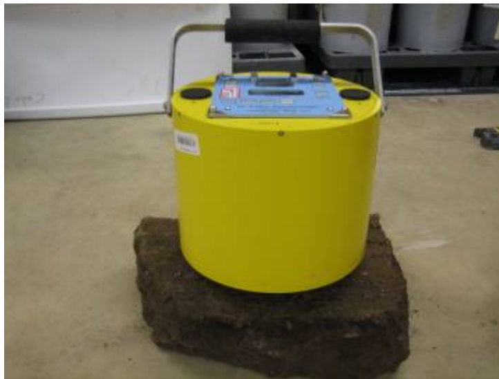
Figure 88. GeoGauge Stiffness Testing.
