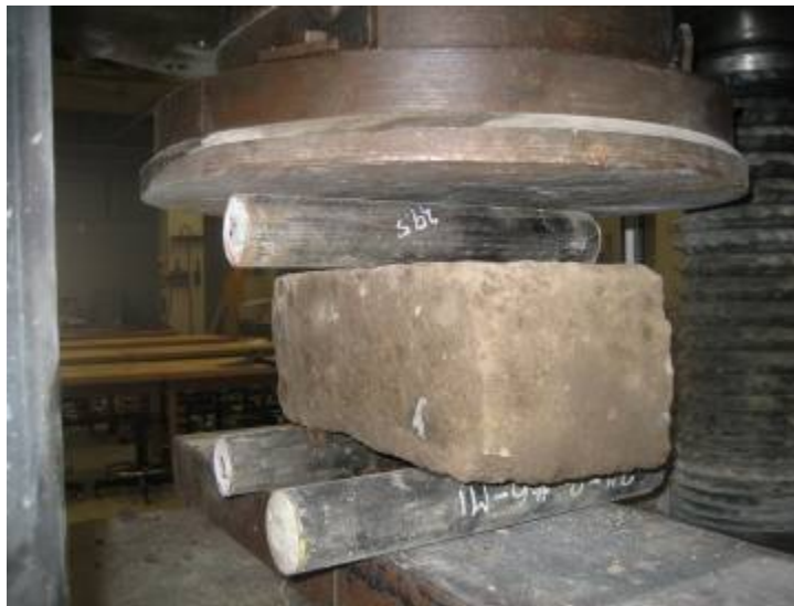
Figure 91. Center Point Flexural Strength Test.
