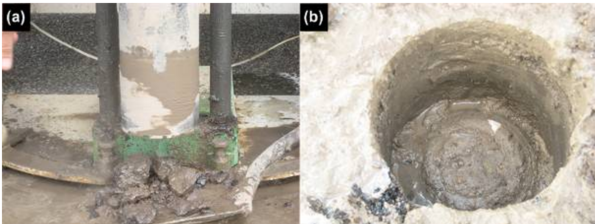
Figure 85. Coring of Field Sample.
