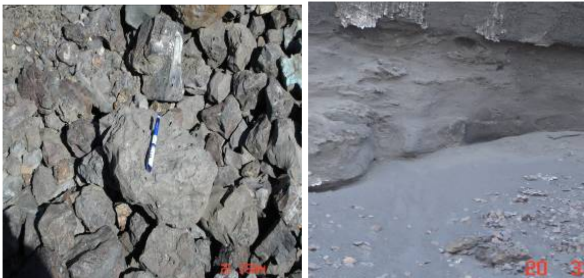
Figure 21. Examples of the Range of Slag Particle Sizes at El Paso Plant.
