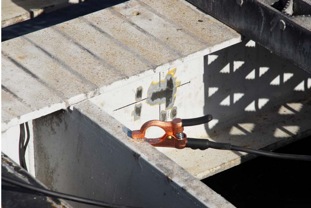
Figure 34. Photograph of Sensor Locations after Grinding.
