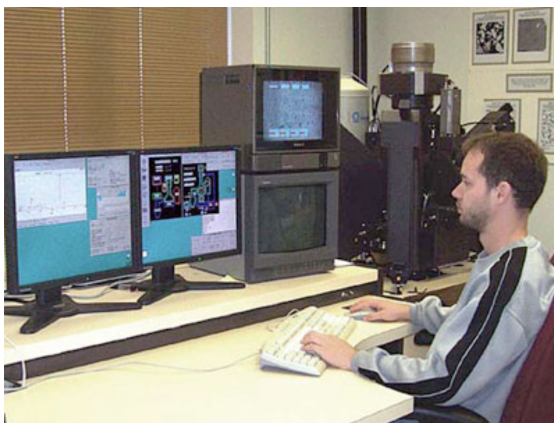
Figure 25. Cameca SX50 Electron Microprobe at Texas A&M University.
