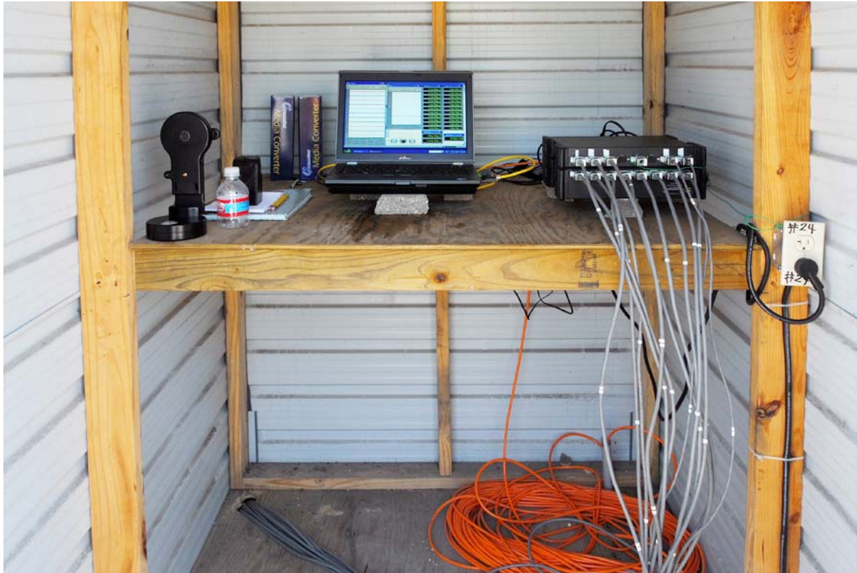
Figure 40. Photograph Showing Data Acquisition System in Out-Building with All Sensors Installed and Operational.
